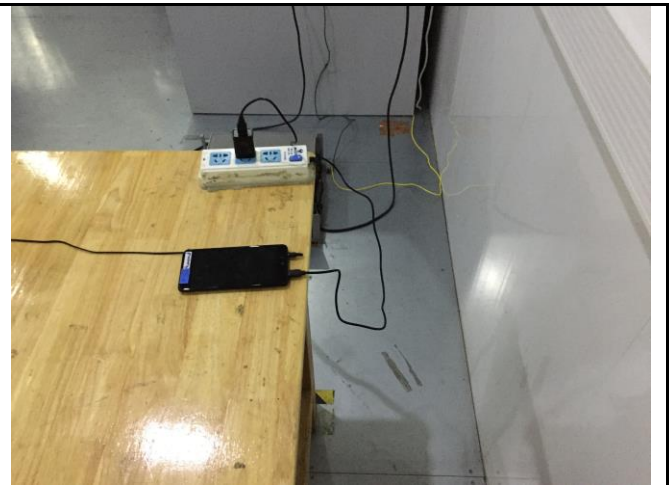
Conducted Emissions Test Setup Side View
