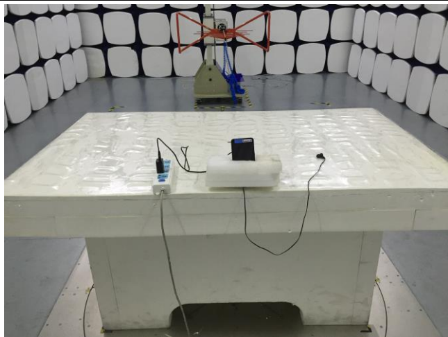
Conducted Emissions Test Setup Front View
