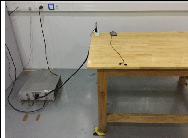
Conducted Emissions Test Setup Front View
