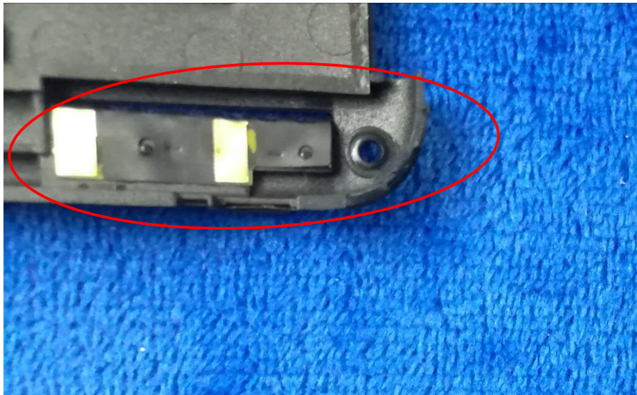
GSM/PCS/UMTS-FDD/LTE Antenna View
