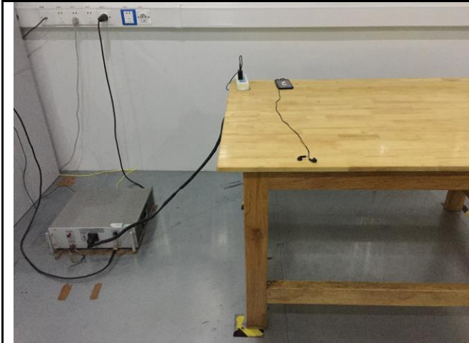
Conducted Emissions Test Setup Front View
