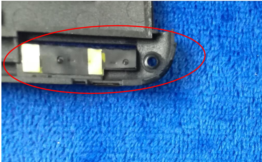
GSM/PCS/UMTS-FDD/LTE Antenna View
