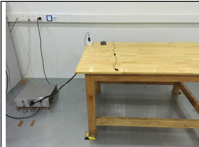
Conducted Emissions Test Setup Front View
