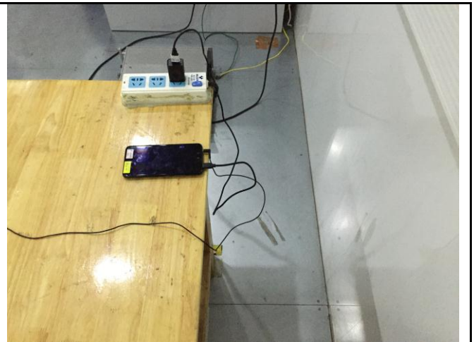
Conducted Emissions Test Setup Side View
