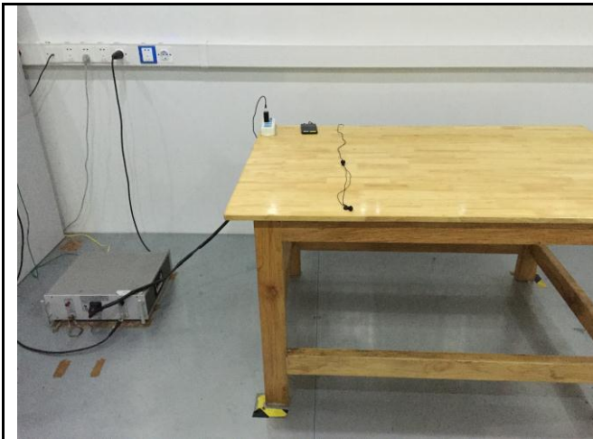
Conducted Emissions Test Setup Front View
