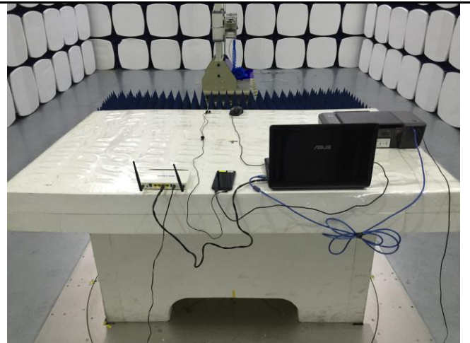
Radiated Emissions Test Setup Above 1GHz
