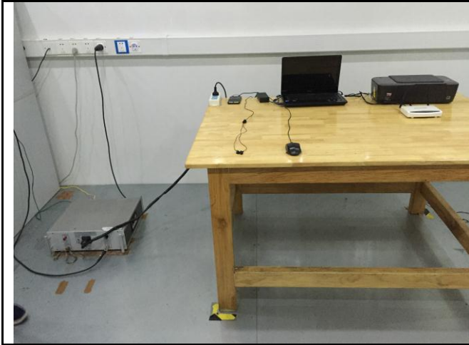
Conducted Emissions Test Setup – Front View
