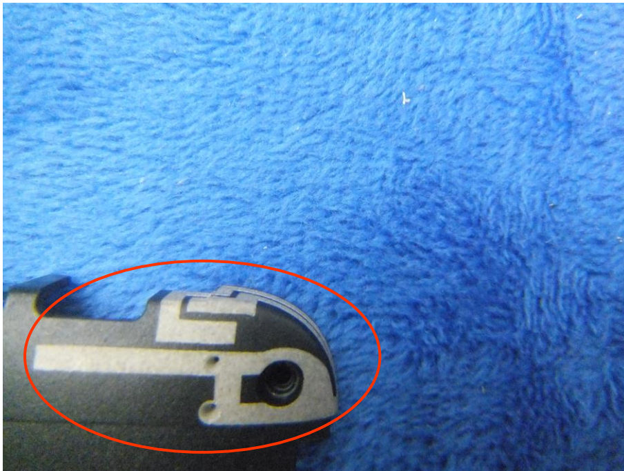
BT/WIFI - Antenna View
