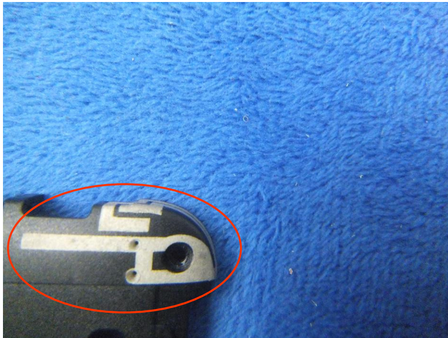
BT/WIFI - Antenna View
