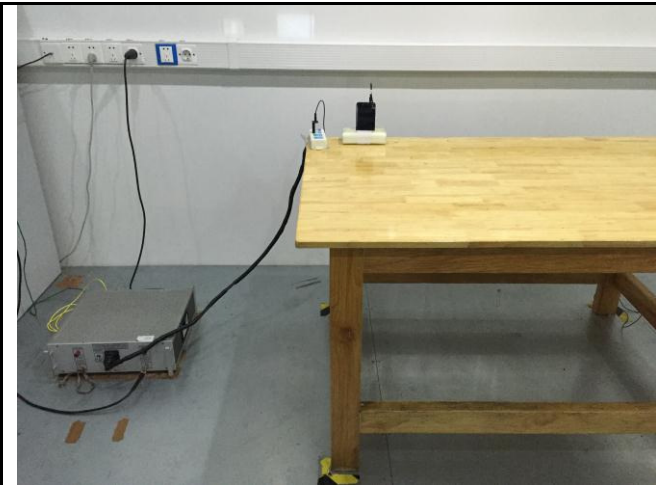
Conducted Emissions Test Setup Front View
