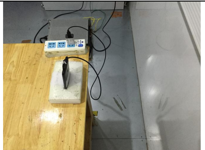
Conducted Emissions Test Setup Side View
