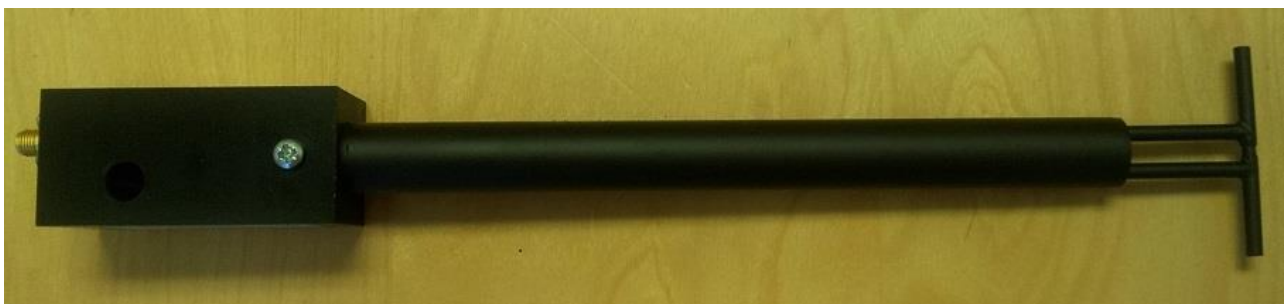
Figure 1 – MVG COMOSAR Validation Dipole
