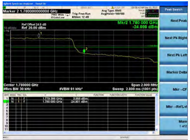
Band66 / 1.4MHz / High CH / QPSK / FULL RB
