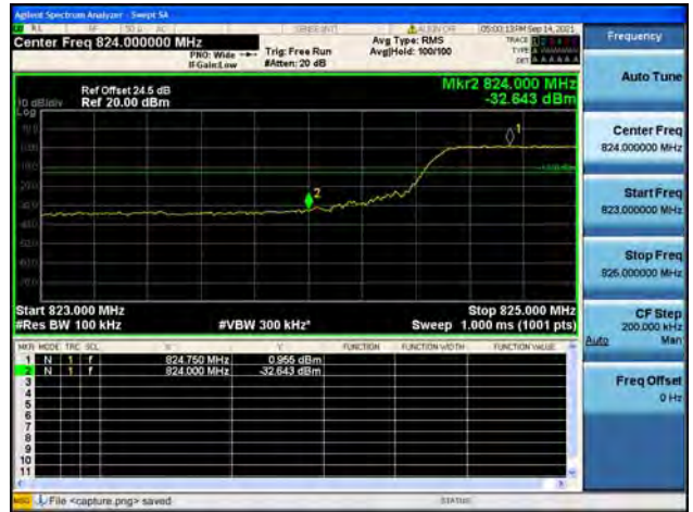
Band5 / 10MHz / High CH / QPSK / FULL RB
