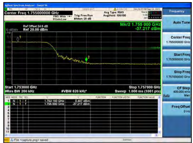
Band4 / 20MHz / High CH / QPSK / FULL RB
