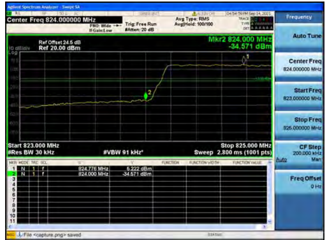
Band5 / 1.4MHz / High CH / QPSK / FULL RB
