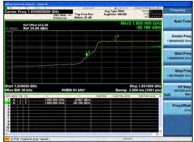
Band2 / 3MHz / High CH / QPSK / FULL RB
