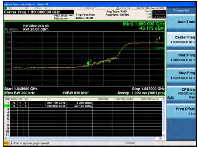
Band2 / 20MHz / High CH / QPSK / FULL RB
