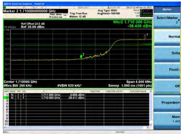
Band66 / 20MHz / High CH / QPSK / FULL RB
