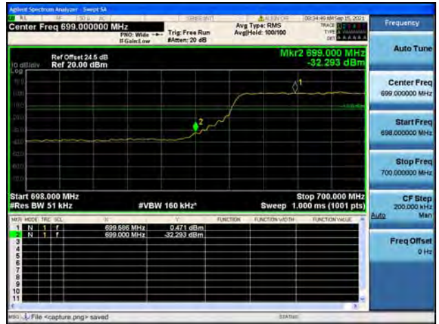
Band12 / 5MHz / High CH / QPSK / FULL RB
