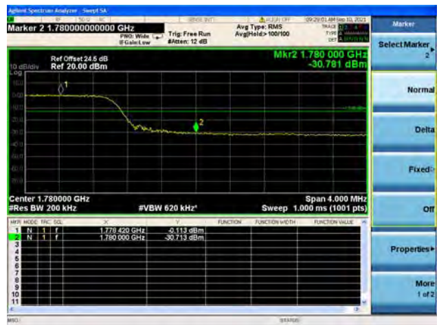
Band66 / 20MHz / High CH / QPSK / FULL RB
