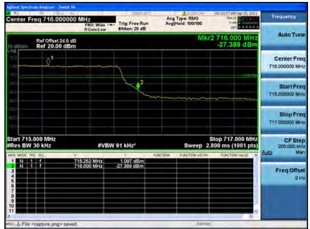
Band12 / 3MHz / High CH / QPSK / FULL RB
