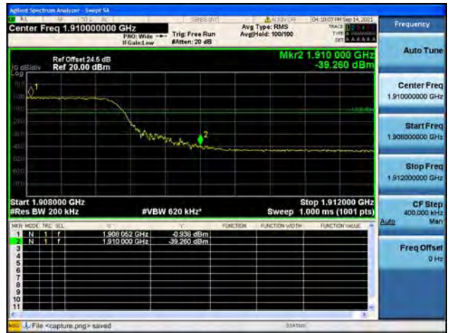
Band2 / 20MHz / High CH / QPSK / FULL RB
