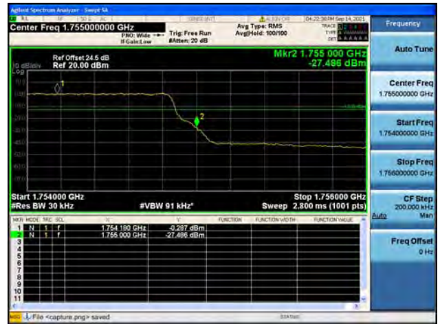
Band4 / 3MHz / High CH / QPSK / FULL RB
