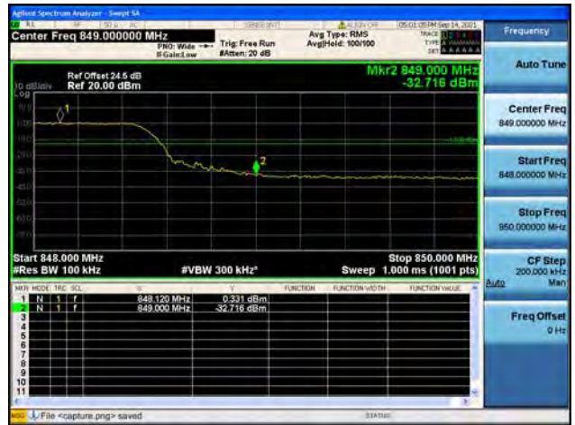
Band5 / 10MHz / High CH / QPSK / FULL RB
