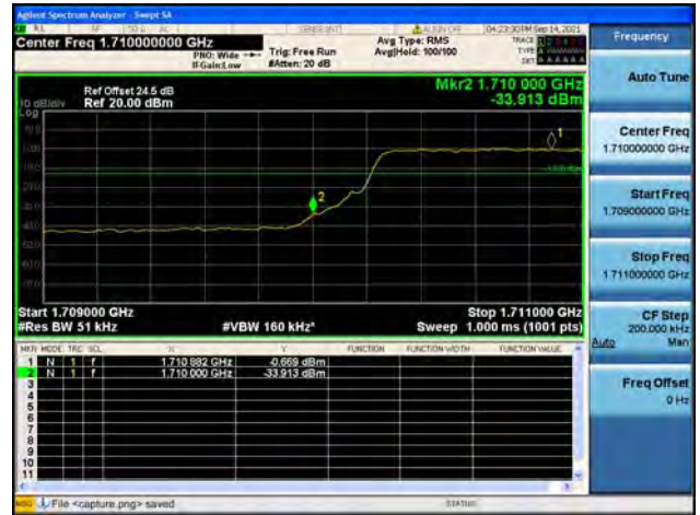
Band4 / 5MHz / High CH / QPSK / FULL RB
