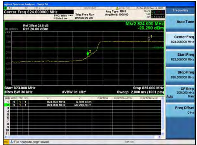
Band5 / 3MHz / High CH / QPSK / FULL RB
