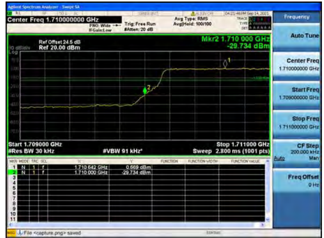
Band4 / 3MHz / High CH / QPSK / FULL RB
