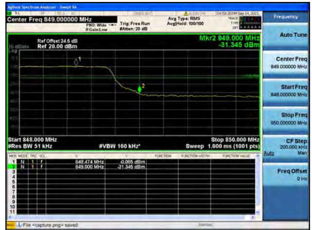
Band5 / 5MHz / High CH / QPSK / FULL RB
