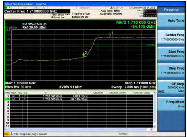
Band4 / 1.4MHz / High CH / QPSK / FULL RB
