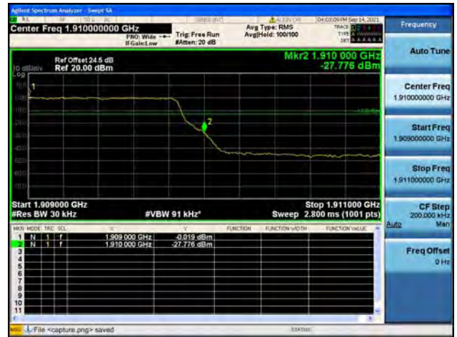
Band2 / 3MHz / High CH / QPSK / FULL RB
