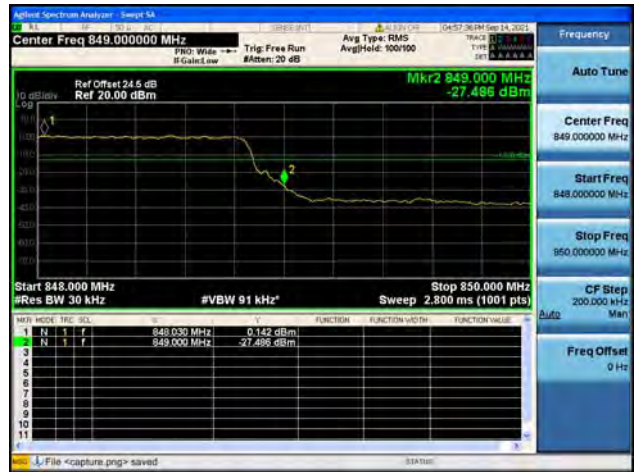
Band5 / 3MHz / High CH / QPSK / FULL RB
