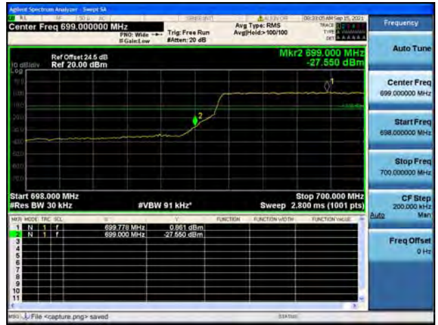
Band12 / 3MHz / High CH / QPSK / FULL RB
