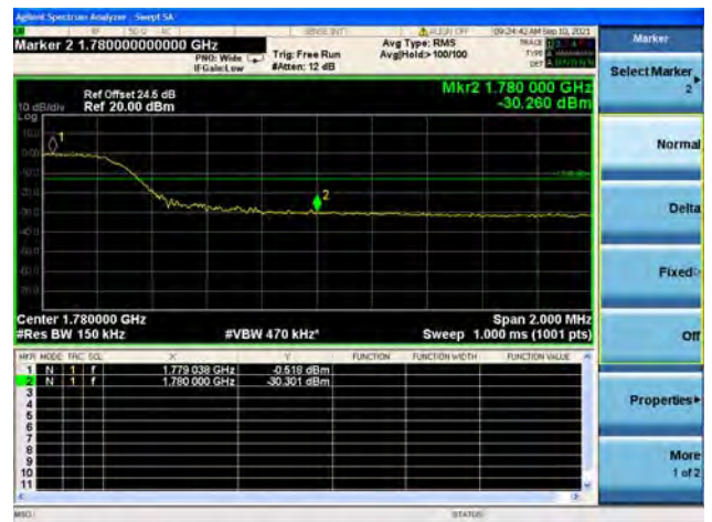
Band66 / 15MHz / High CH / QPSK / FULL RB
