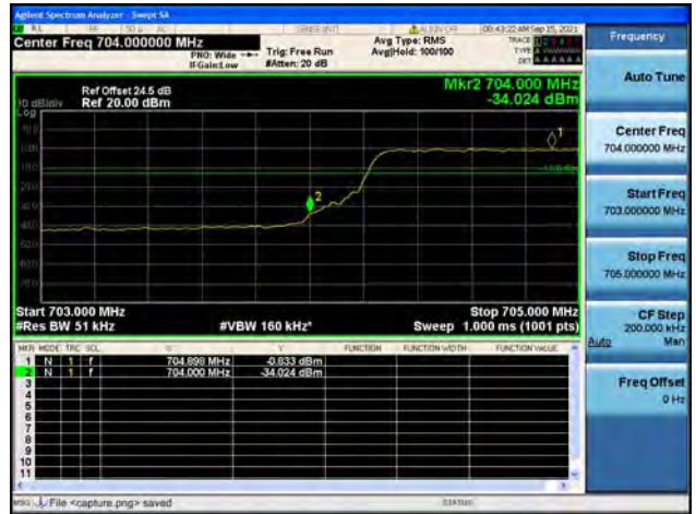
Band17 / 5MHz / High CH / QPSK / FULL RB
