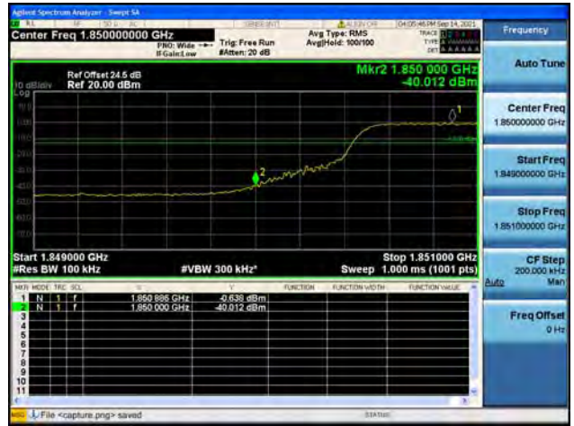
Band2 / 10MHz / High CH / QPSK / FULL RB
