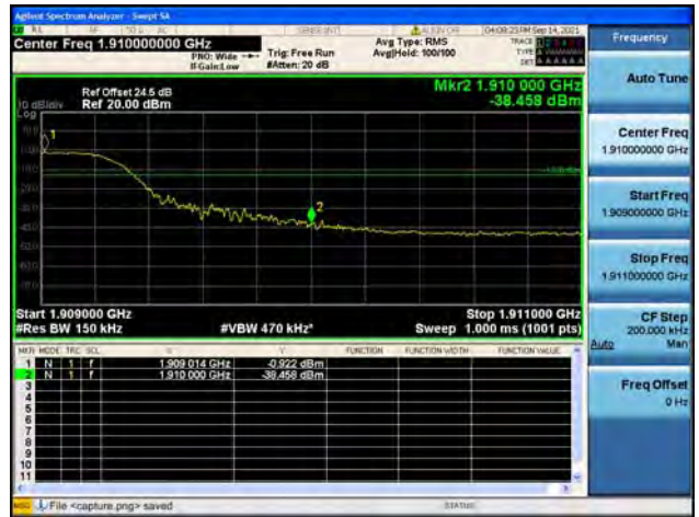
Band2 / 15MHz / High CH / QPSK / FULL RB
