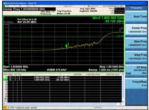
Band2 / 15MHz / High CH / QPSK / FULL RB
