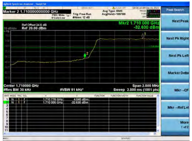
Band66 / 1.4MHz / High CH / QPSK / FULL RB
