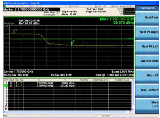
Band66 / 10MHz / High CH / QPSK / FULL RB
