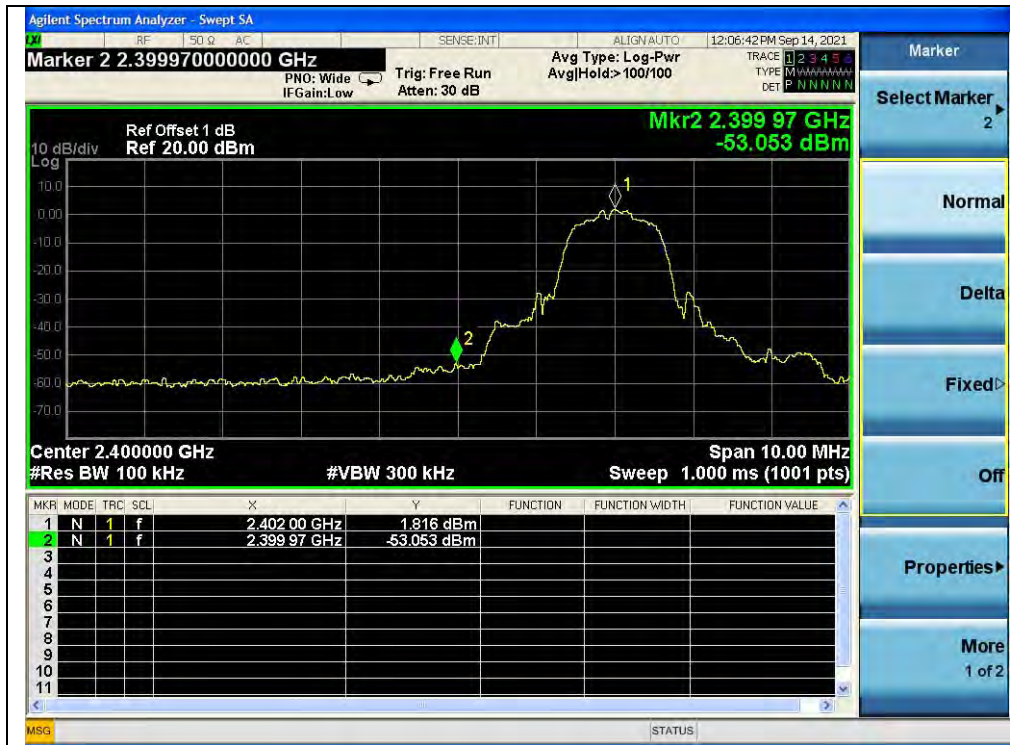
(Band edge, Channel 0, \pi/4 -DQPSK)
