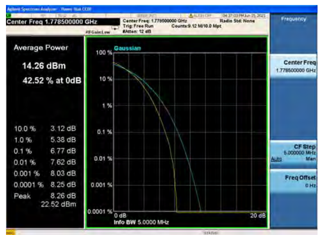
Band66 / 3MHz / High CH / 64QAM
