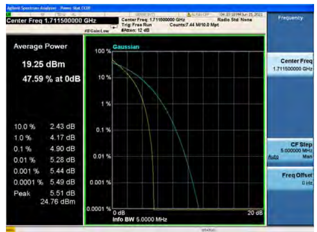
Band66 / 3MHz / Low CH / 64QAM
