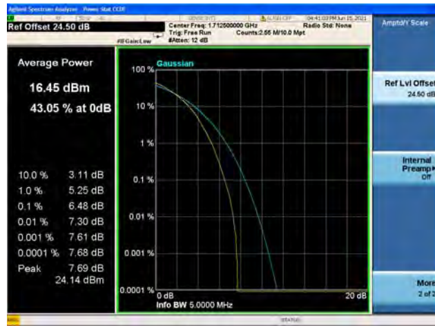
Band66 / 5MHz / Mid CH / 16QAM
