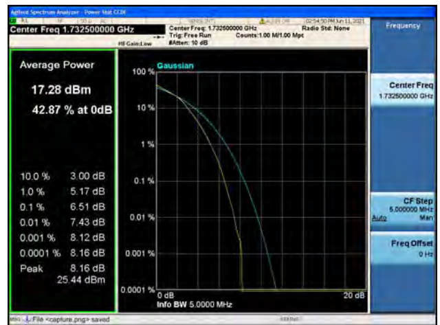
Band4 / 5MHz / Mid CH / 64QAM
