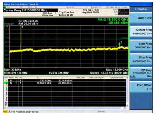
Band4 / 5MHz / Mid CH / 64QAM
