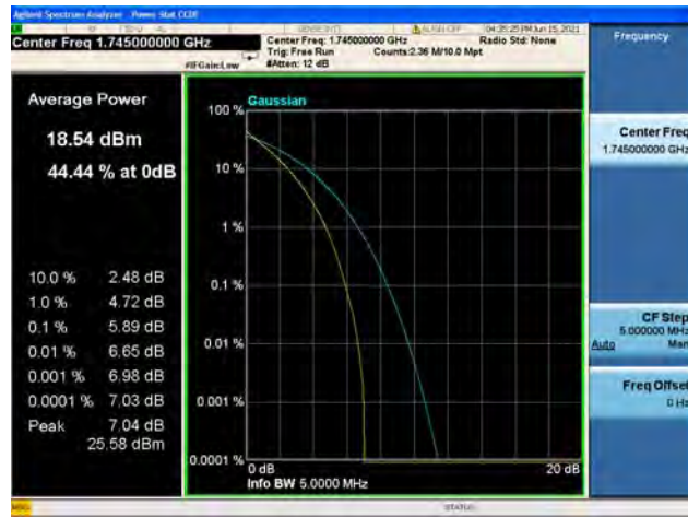
Band66 / 3MHz / Mid CH / 64QAM
