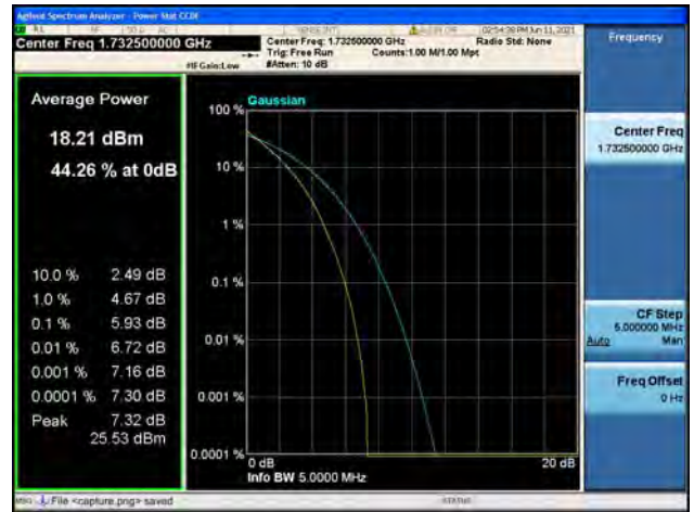
Band4 / 5MHz / Mid CH / 64QAM
