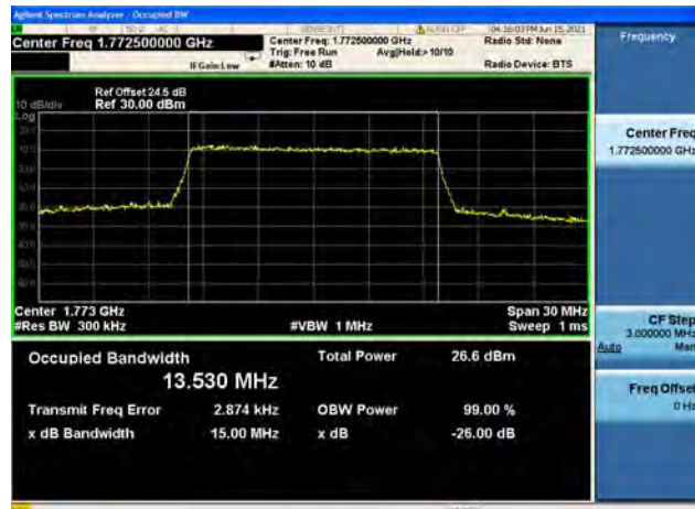
Band66 / 15MHz / High CH / 64QAM
