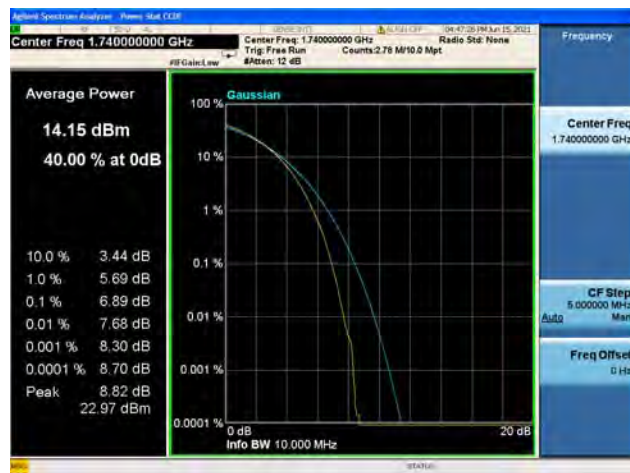
Band66 / 10MHz / High CH / 16QAM
