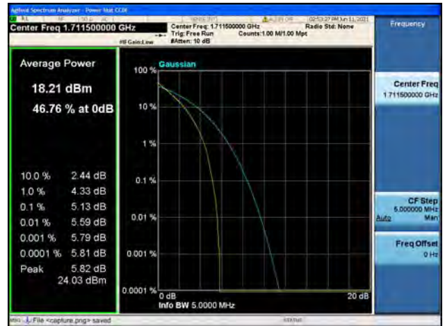
Band4 / 3MHz / Low CH / 64QAM
