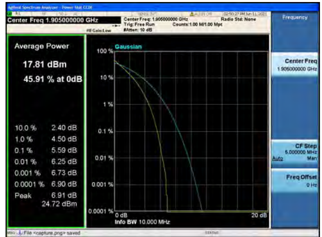
Band2 / 10MHz / High CH / 64QAM
