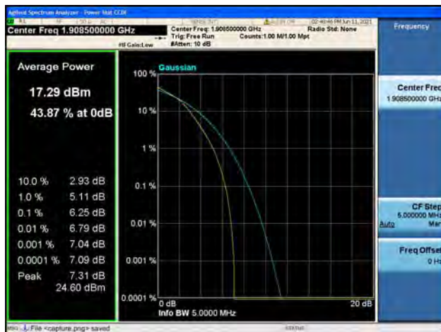
Band2 / 3MHz / High CH / 16QAM
