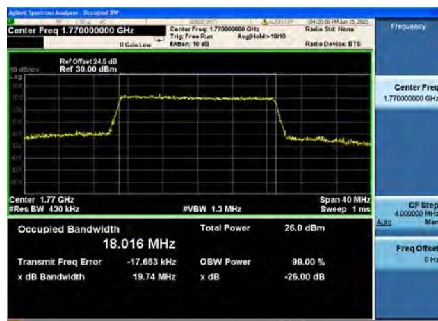
Band66 / 20MHz / High CH / 16QAM
