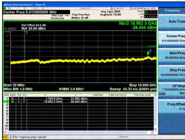
Band4 / 1.4MHz / High CH / 64QAM
