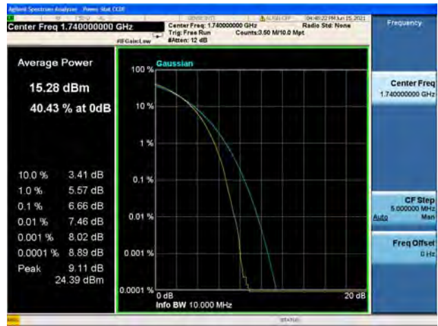
Band66 / 10MHz / High CH / QPSK
