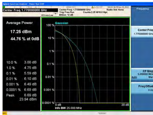
Band66 / 20MHz / High CH / 16QAM
