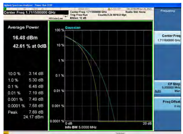
Band66 / 3MHz / Low CH / 64QAM
