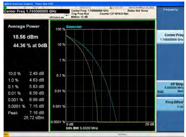
Band66 / 5MHz / Mid CH / 64QAM
