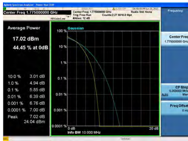
Band66 / 10MHz / High CH / 16QAM
