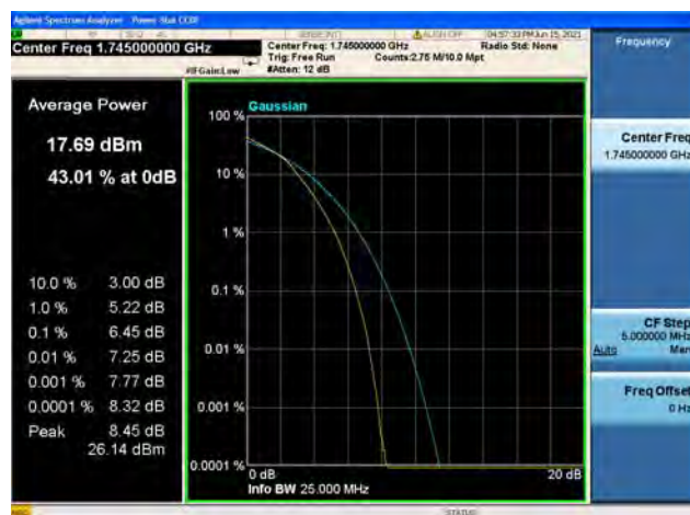
Band66 / 15MHz / Mid CH / 16QAM
