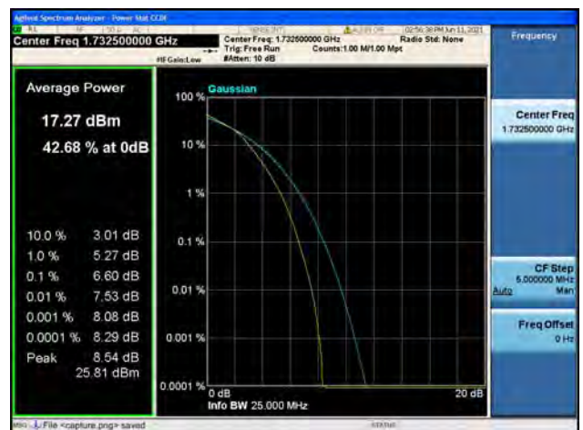
Band4 / 15MHz / Mid CH / 64QAM
