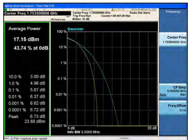
Band4 / 3MHz / High CH / 64QAM
