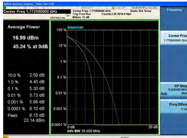
Band66 / 15MHz / High CH / 64QAM
