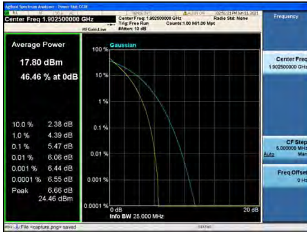
Band2 / 15MHz / High CH / 64QAM
