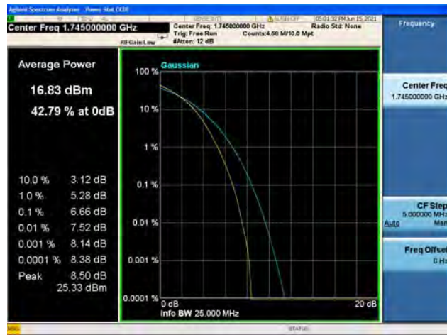
Band66 / 20MHz / High CH / 16QAM
