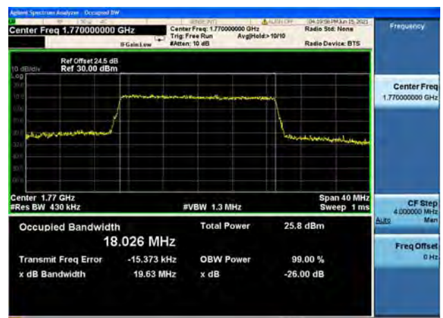
Band66 / 20MHz / High CH / 64QAM
