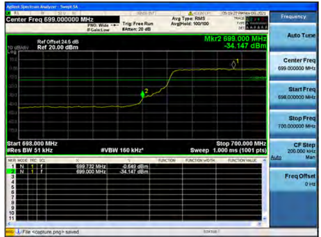
Band12 / 5MHz / High CH / QPSK / FULL RB
