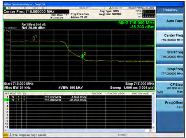
Band12 / 5MHz / High CH / QPSK / FULL RB
