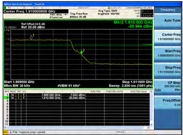
Band2 / 3MHz / High CH / QPSK / FULL RB
