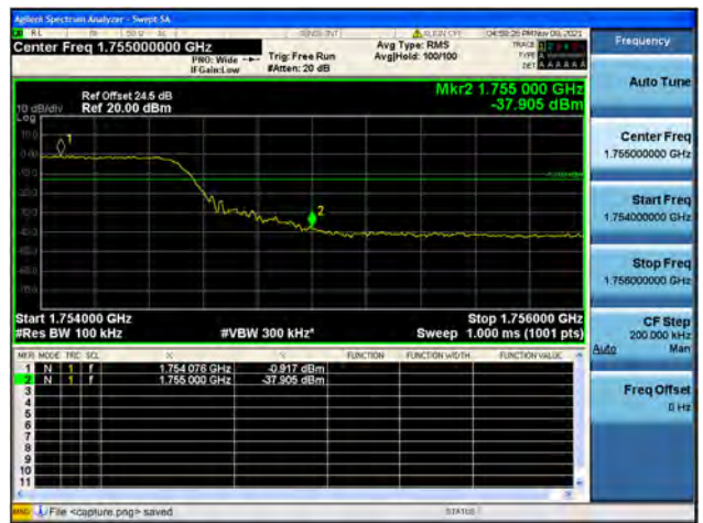
Band4 / 10MHz / High CH / QPSK / FULL RB
