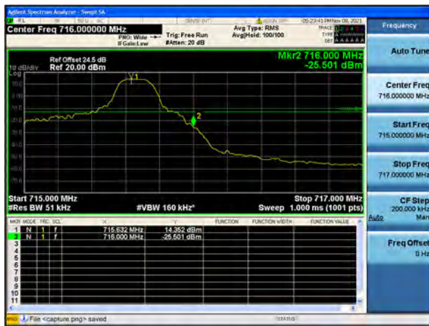
Band17 / 5MHz / High CH / QPSK / 1 RB
