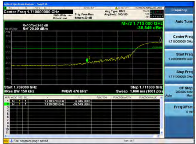
Band4 / 15MHz / High CH / QPSK / FULL RB
