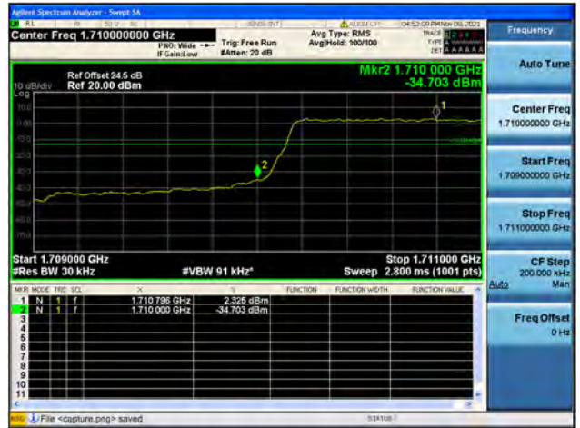
Band4 / 1.4MHz / High CH / QPSK / FULL RB
