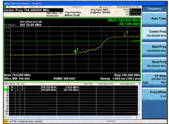
Band17 / 10MHz / High CH / QPSK / FULL RB
