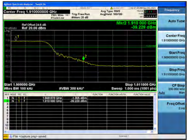
Band2 / 10MHz / High CH / QPSK / FULL RB
