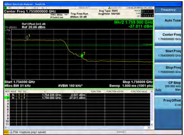
Band4 / 5MHz / High CH / QPSK / FULL RB
