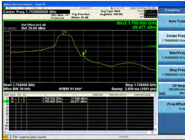
Band4 / 1.4MHz / High CH / QPSK / 1 RB
