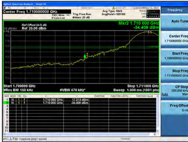
Band66 / 15MHz / High CH / QPSK / 1 RB
