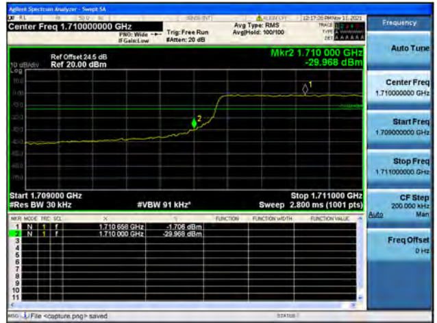
Band66 / 3MHz / High CH / QPSK / FULL RB
