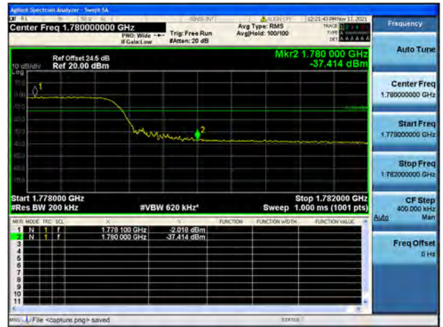
Band66 / 20MHz / High CH / QPSK / FULL RB
