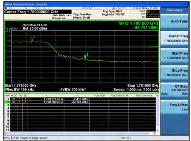
Band66 / 10MHz / High CH / QPSK / FULL RB
