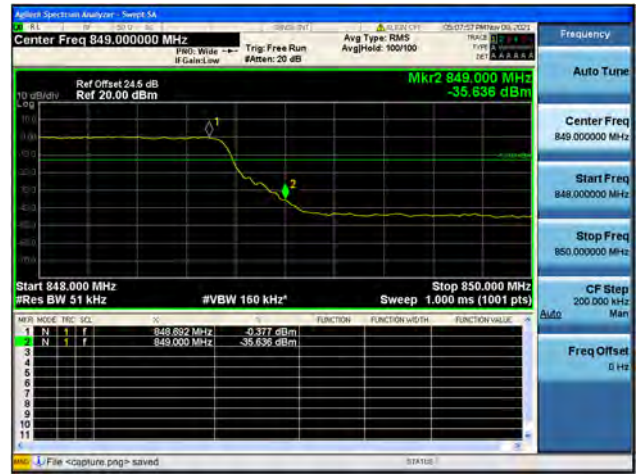
Band5 / 5MHz / High CH / QPSK / FULL RB
