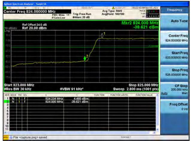
Band5 / 1.4MHz / High CH / QPSK / FULL RB
