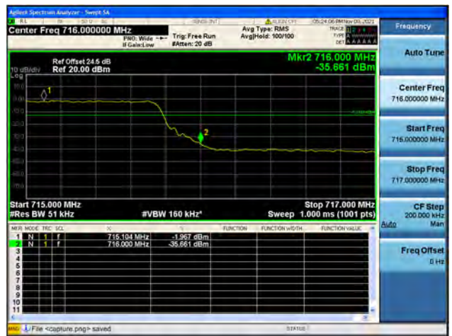
Band17 / 5MHz / High CH / QPSK / FULL RB
