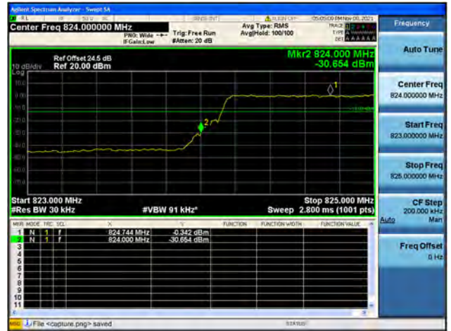
Band5 / 3MHz / High CH / QPSK / FULL RB
