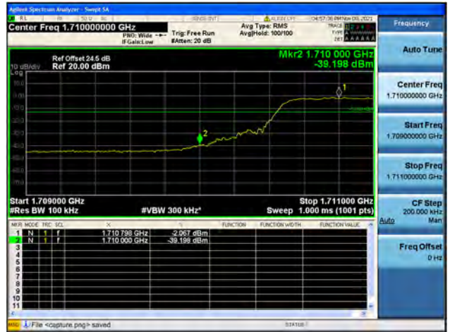
Band4 / 10MHz / High CH / QPSK / FULL RB
