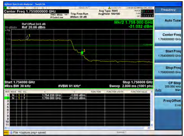
Band4 / 3MHz / High CH / QPSK / FULL RB
