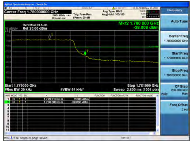
Band66 / 1.4MHz / High CH / QPSK / FULL RB
