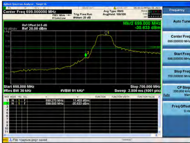
Band12 / 1.4MHz / High CH / QPSK / 1 RB
