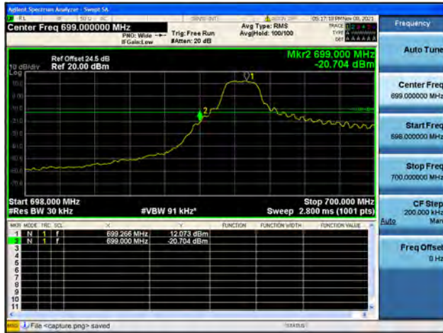
Band12 / 3MHz / High CH / QPSK / 1 RB
