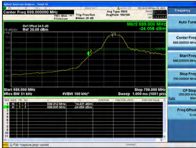
Band12 / 5MHz / High CH / QPSK / 1 RB
