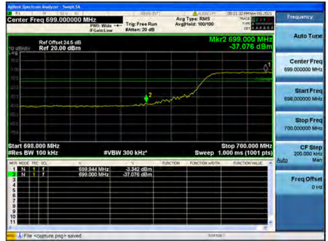
Band12 / 10MHz / High CH / QPSK / FULL RB
