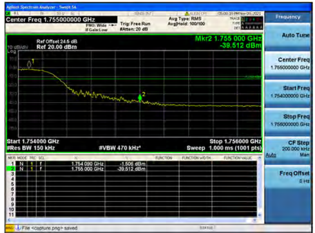
Band4 / 15MHz / High CH / QPSK / FULL RB
