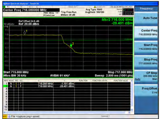
Band12 / 3MHz / High CH / QPSK / FULL RB
