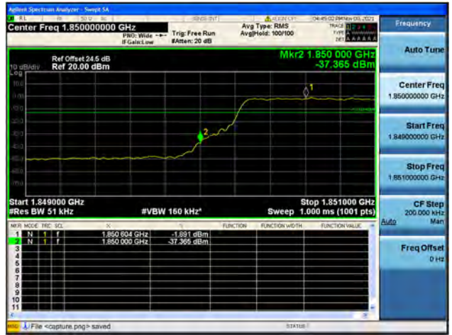
Band2 / 5MHz / High CH / QPSK / FULL RB
