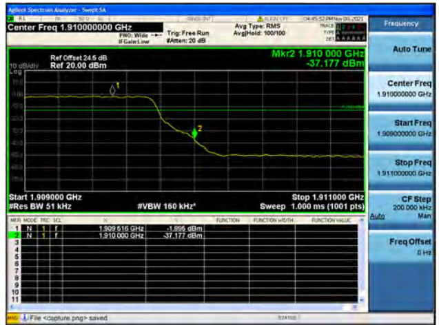
Band2 / 5MHz / High CH / QPSK / FULL RB
