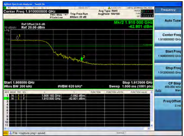
Band2 / 20MHz / High CH / QPSK / FULL RB
