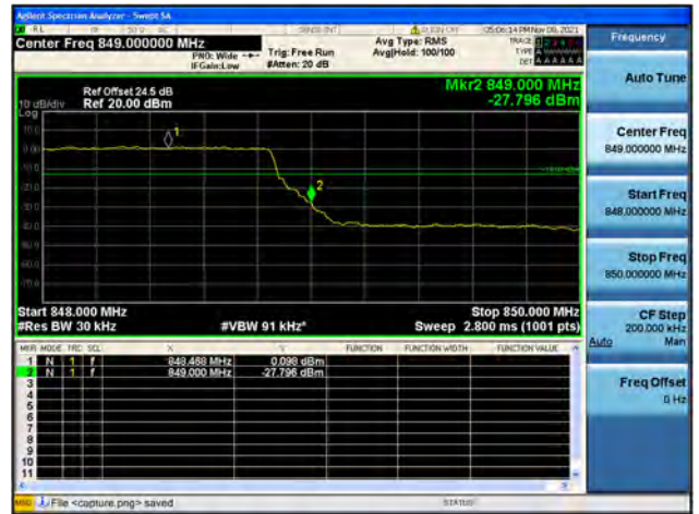
Band5 / 3MHz / High CH / QPSK / FULL RB
