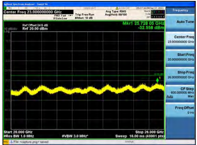
Band7-20G-26G / 20MHz / High CH / 16QAM
