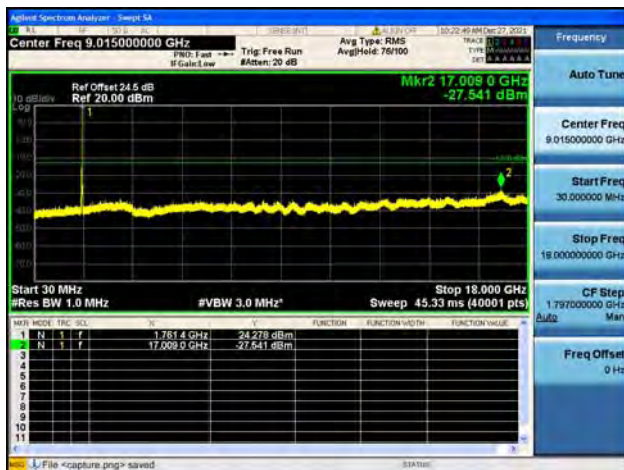
Band66 / 20MHz / High CH / 16QAM
