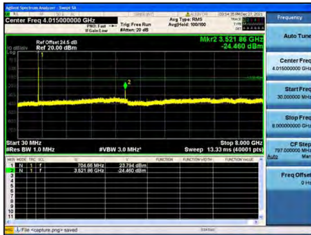
Band17 / 5MHz / Low CH / 64QAM
