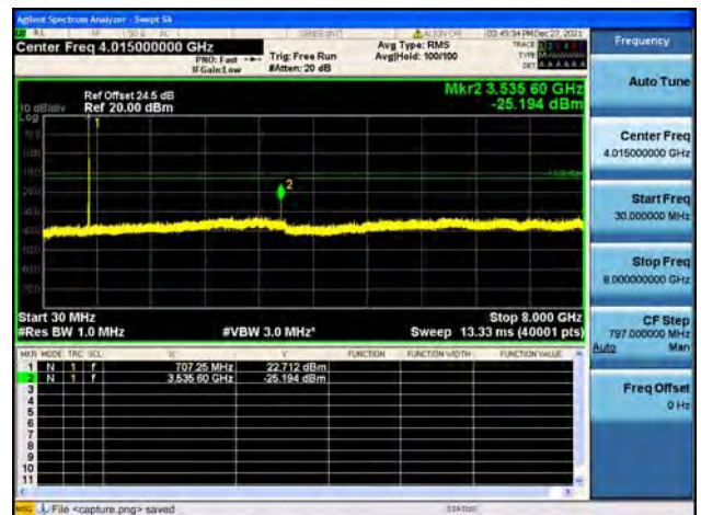
Band12 / 1.4MHz / Mid CH / 64QAM
