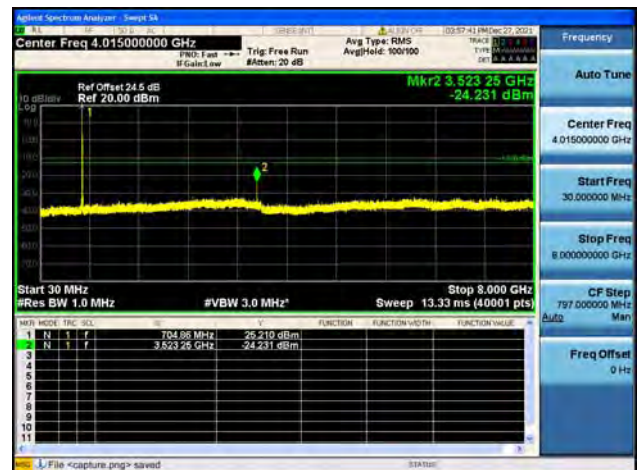
Band17 / 10MHz / Low CH / 64QAM
