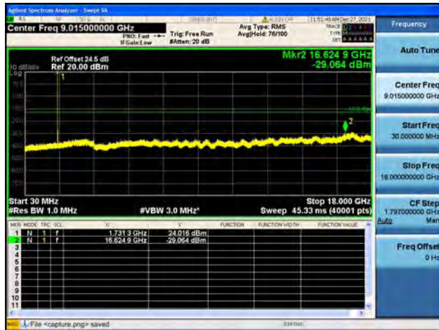
Band4 / 3MHz / High CH / 16QAM
