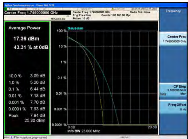
Band66 / 15MHz / Mid CH / 64QAM
