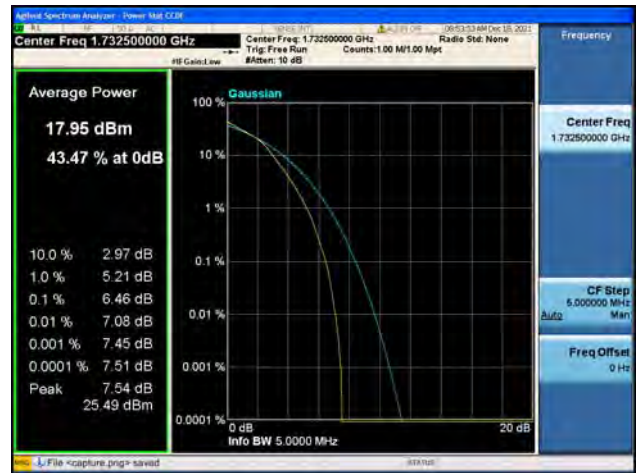
Band4 / 3MHz / High CH / QPSK
