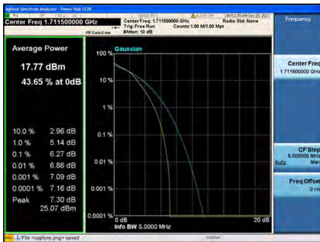
Band4 / 3MHz / Low CH / 16QAM
