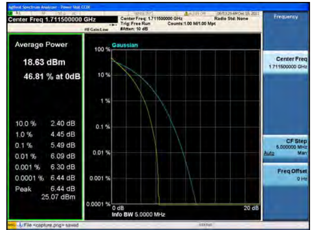
Band4 / 3MHz / Low CH / 64QAM
