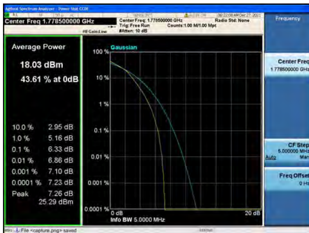
Band66 / 3MHz / High CH / 16QAM
