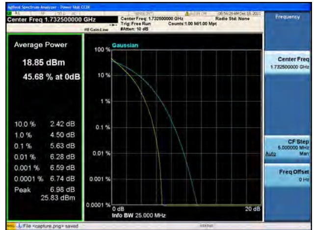
Band4 / 15MHz / Mid CH / 64QAM
