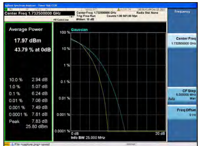
Band4 / 15MHz / Mid CH / 64QAM
