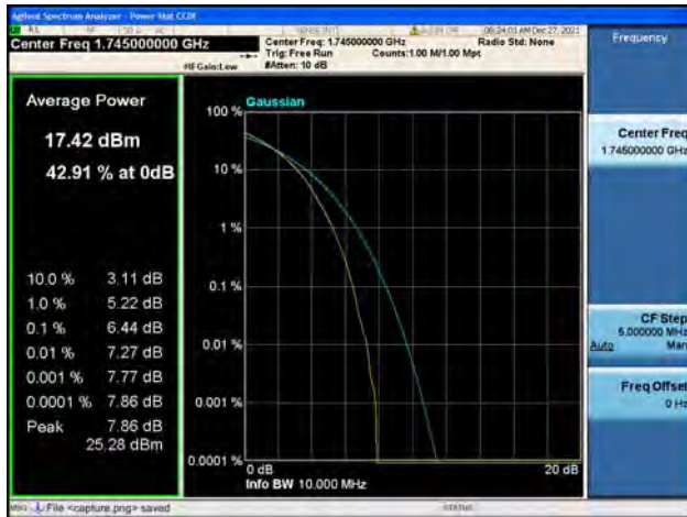
Band66 / 10MHz / High CH / 16QAM
