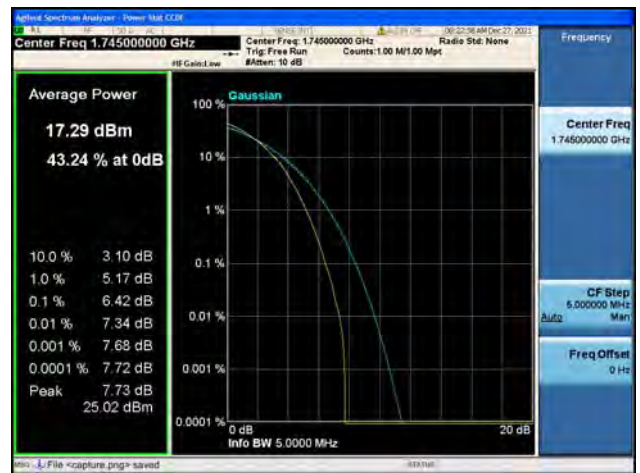
Band66 / 5MHz / Mid CH / 64QAM
