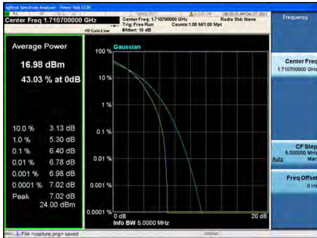
Band66 / 1.4MHz / Mid CH / 16QAM
