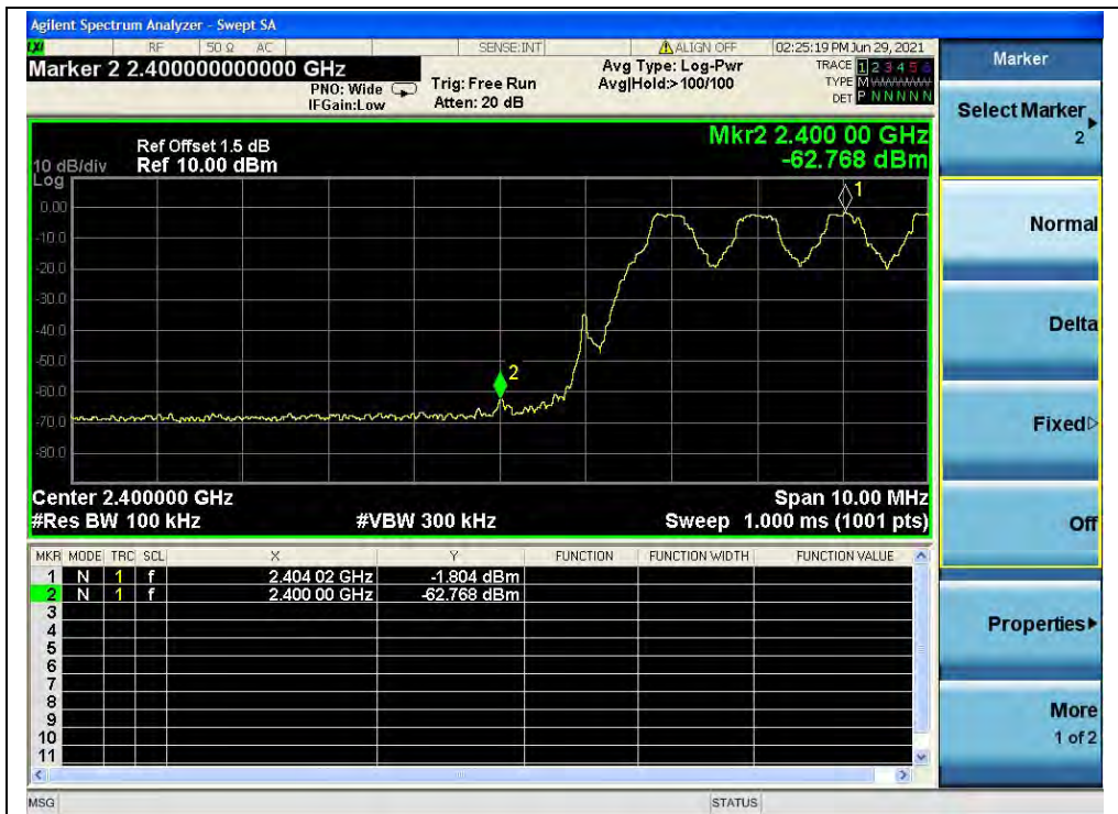
(Band edge with hopping on, Channel 0, GFSK)
