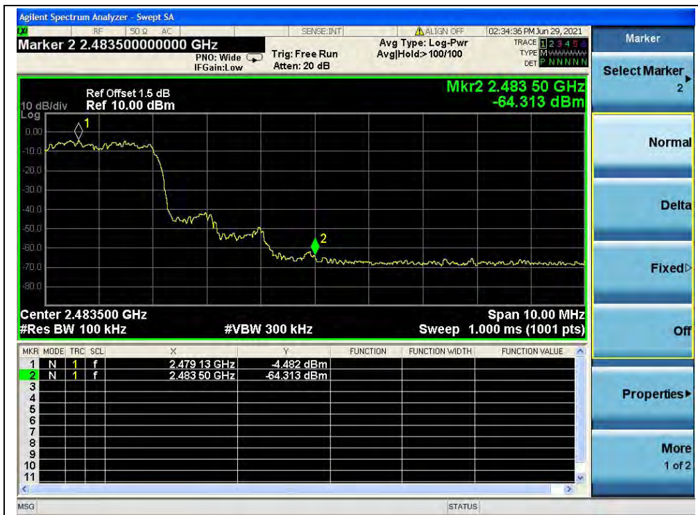
(Band edge with hopping on, Channel 78, 8-DPSK)
