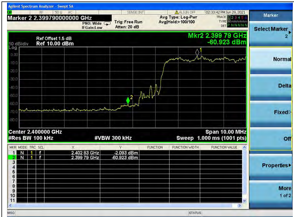
(Band edge with hopping on, Channel 0, 8-DPSK)
