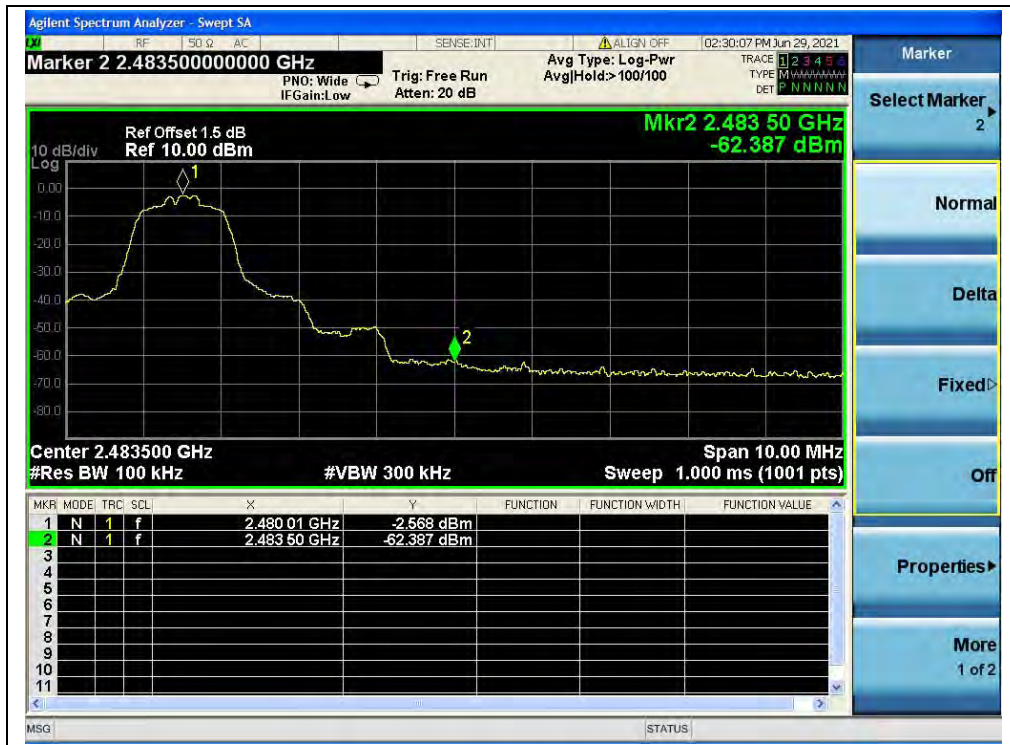
(Band edge, Channel 78, \pi/4 -DQPSK)
