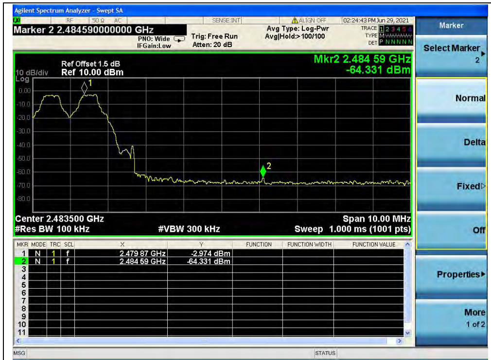
(Band edge with hopping on, Channel 78, GFSK)
