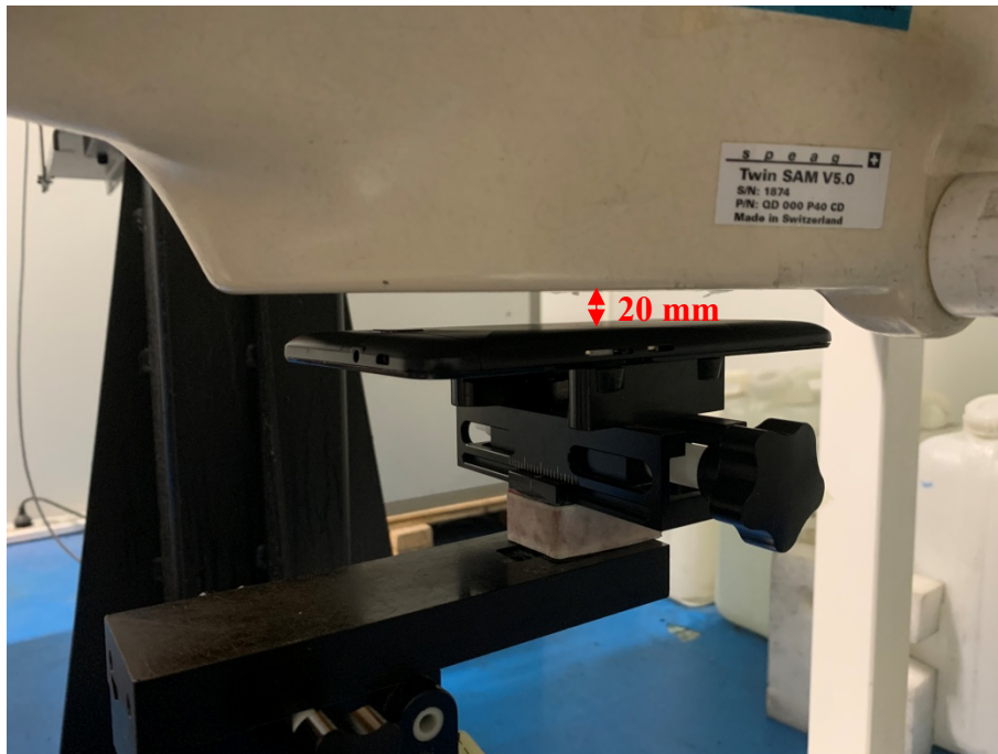
Body (Worn) Back Setup Photo (20mm)
