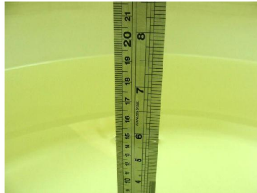
Fig 7.2 Photo of Liquid Height for Body SAR
