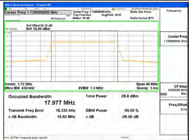
Band66 / 20MHz / 64QAM/ Low CH
