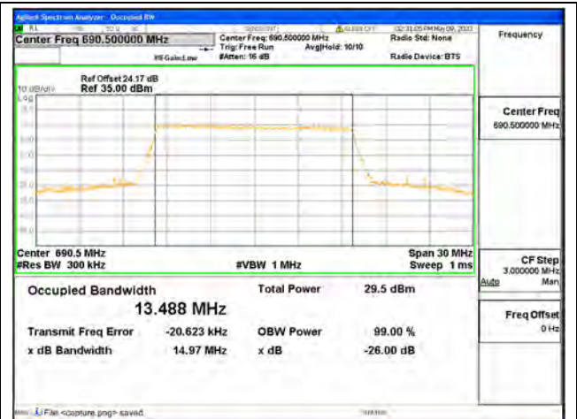
Band71 / 15MHz / 16QAM/ High CH
