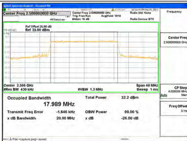
Band41 / 20MHz / 16QAM/ Low CH
