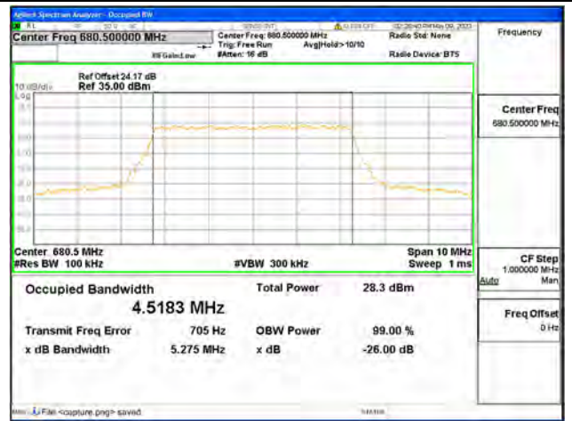
Band71 / 5MHz / 64QAM/ Mid CH
