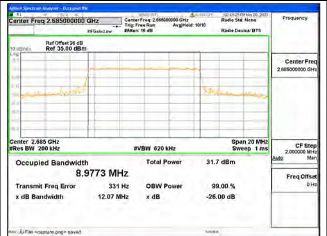
Band41 / 10MHz / 64QAM/ High CH
