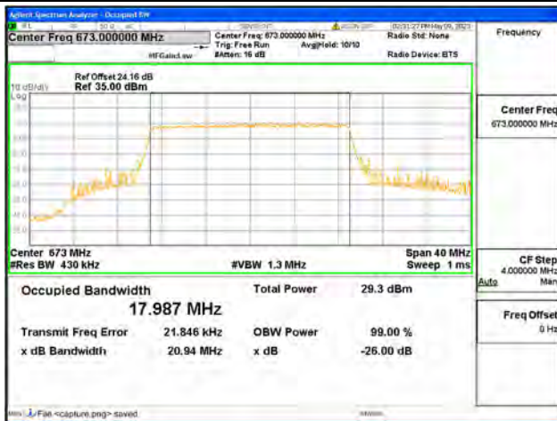
Band71 / 20MHz / 16QAM/ Low CH
