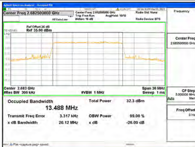
Band41 / 15MHz / 64QAM/ High CH
