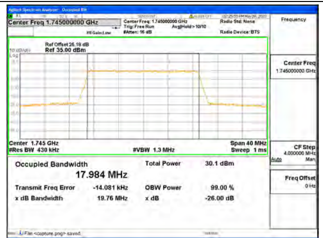
Band66 / 20MHz / 16QAM/ Mid CH
