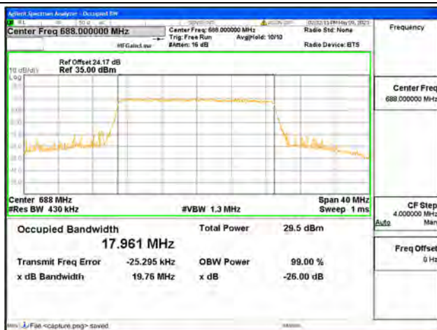
Band71 / 20MHz / 16QAM/ High CH
