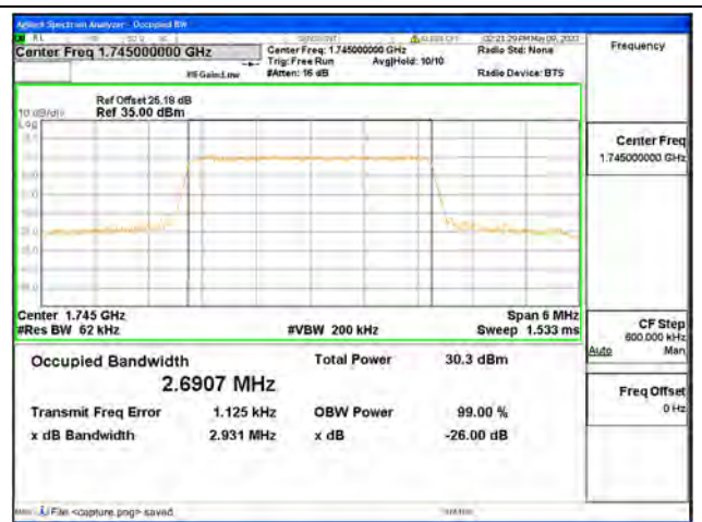
Band66 / 3MHz / 16QAM/ Mid CH
