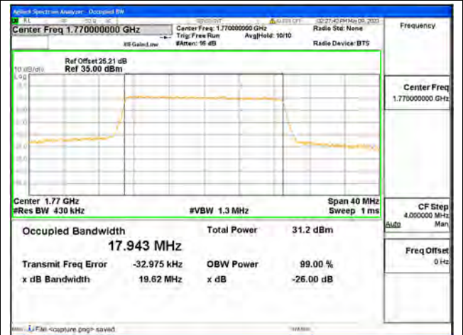
Band66 / 20MHz / QPSK/ High CH
