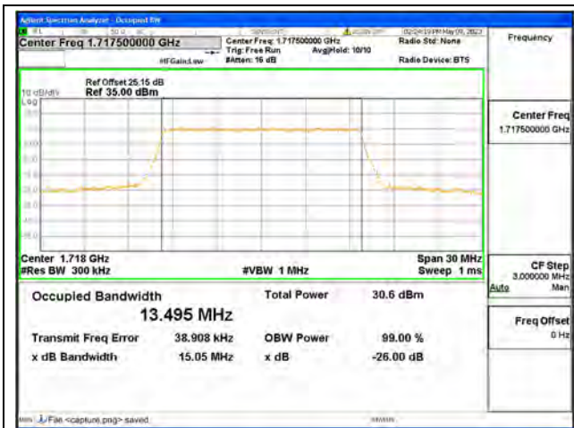
Band66 / 15MHz / QPSK/ Low CH
