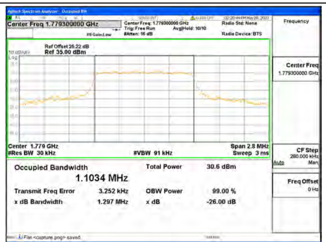
Band66 / 1.4MHz / 16QAM/ High CH
