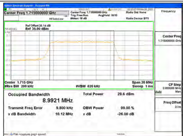
Band66 / 10MHz / 64QAM/ Low CH
