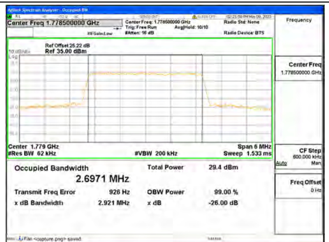
Band66 / 3MHz / 64QAM/ High CH
