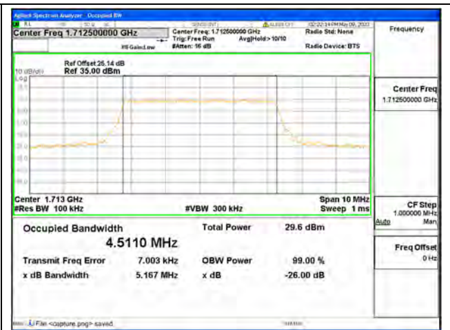
Band66 / 5MHz / 16QAM/ Low CH
