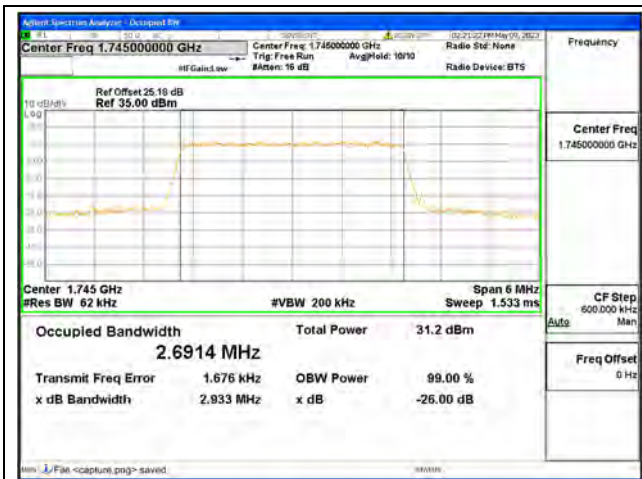
Band66 / 3MHz / QPSK/ Mid CH
