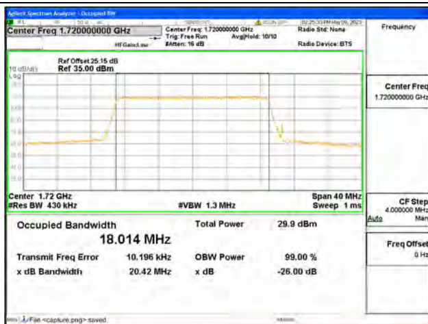
Band66 / 20MHz / 16QAM/ Low CH
