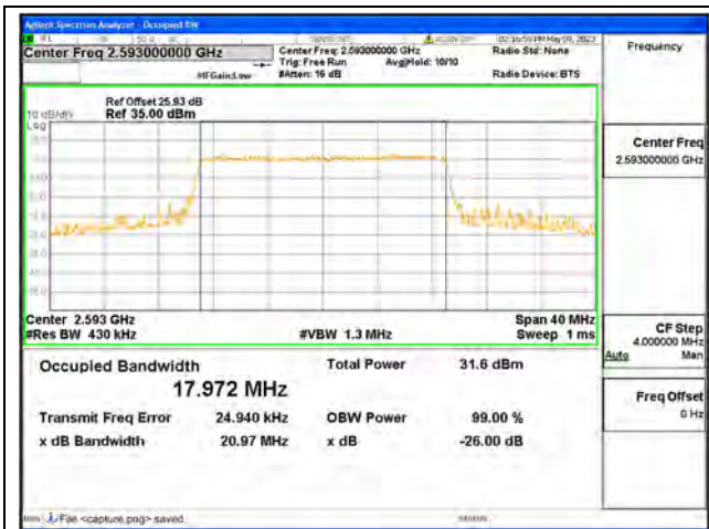
Band41 / 20MHz / QPSK/ Mid CH
