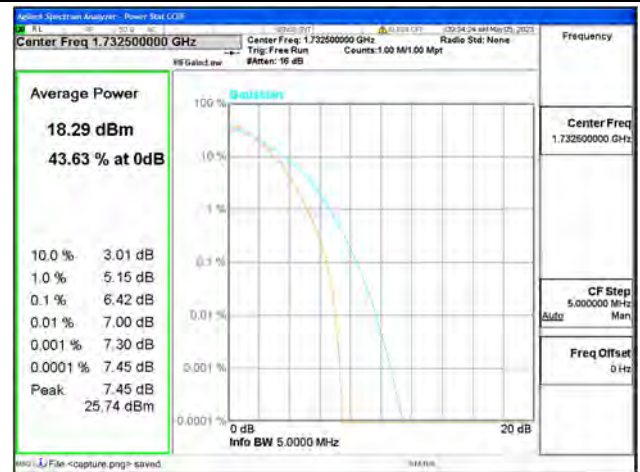
Band4 / 1.4MHz / Mid CH / 64QAM
