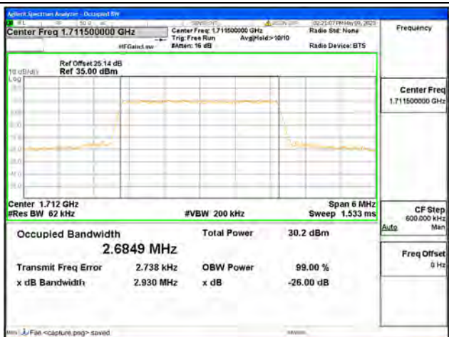
Band66 / 3MHz / 16QAM/ Low CH
