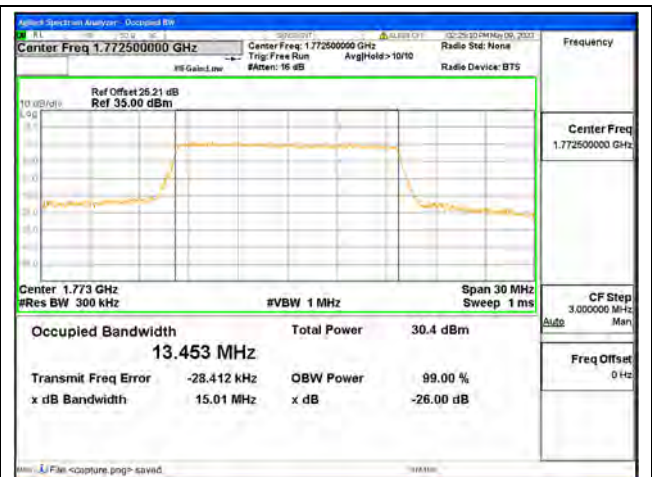
Band66 / 15MHz / 16QAM/ High CH
