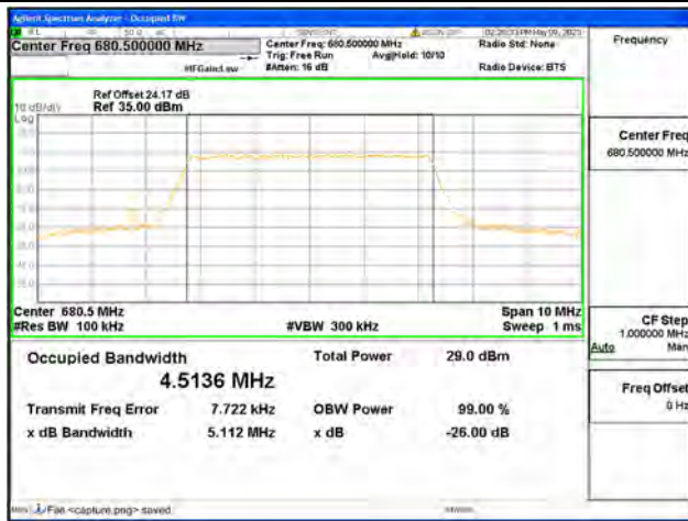
Band71 / 5MHz / 16QAM/ Mid CH
