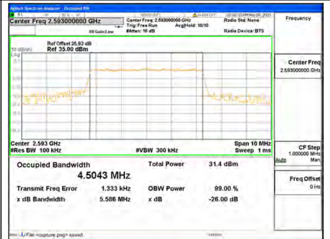
Band41 / 5MHz / QPSK/ Mid CH
