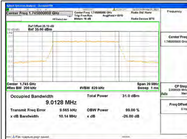
Band66 / 10MHz / QPSK/ Mid CH
