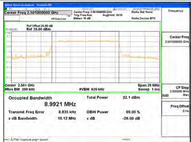
Band41 / 10MHz / QPSK/ Low CH
