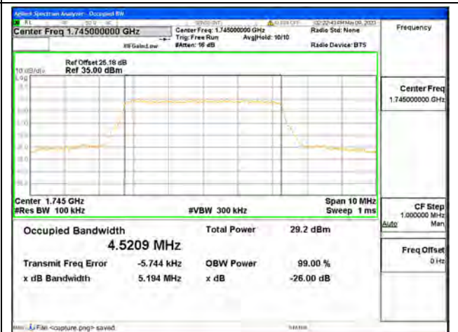
Band66 / 5MHz / 64QAM/ Mid CH
