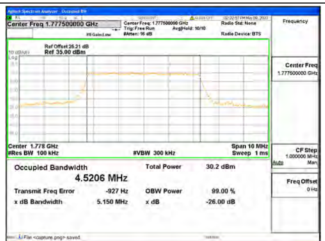
Band66 / 5MHz / 16QAM/ High CH
