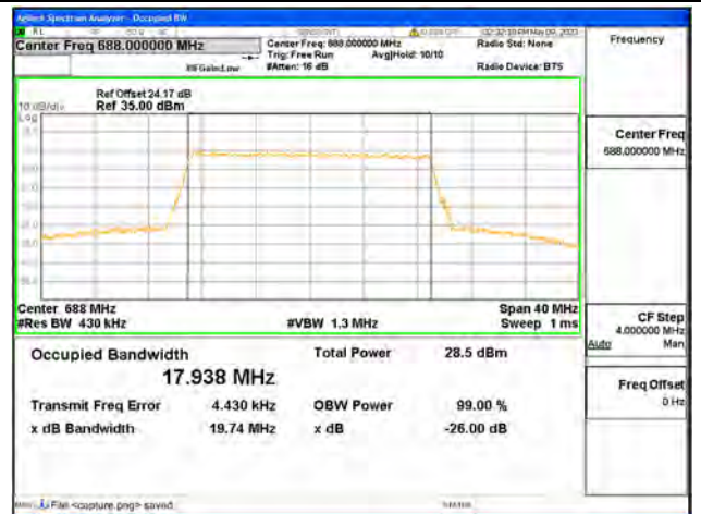
Band71 / 20MHz / 64QAM/ High CH
