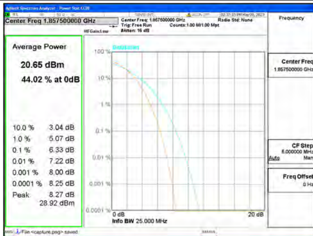
Band25 / 15MHz / Low CH / 64QAM
