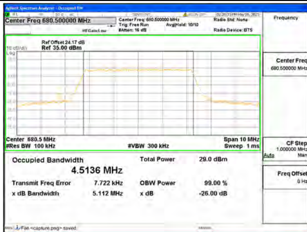
Band71 / 5MHz / 16QAM/ Mid CH
