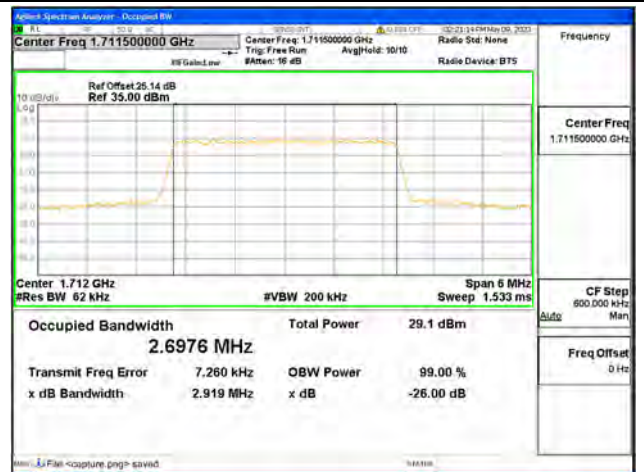
Band66 / 3MHz / 64QAM/ Low CH
