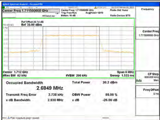
Band66 / 3MHz / 16QAM/ Low CH
