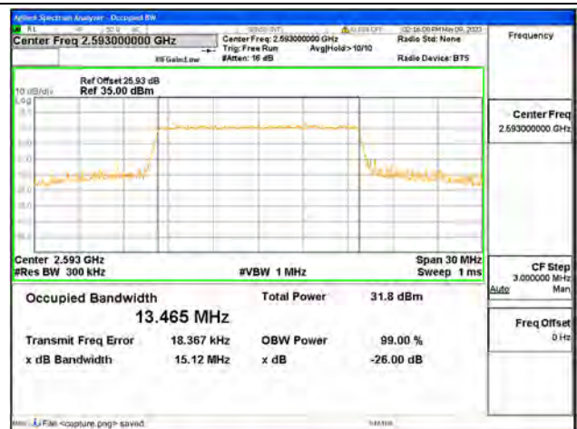
Band41 / 15MHz / 64QAM/ Mid CH
