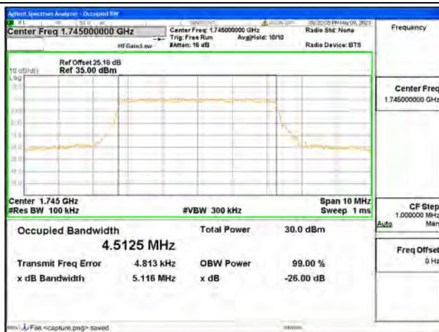
Band66 / 5MHz / 16QAM/ Mid CH
