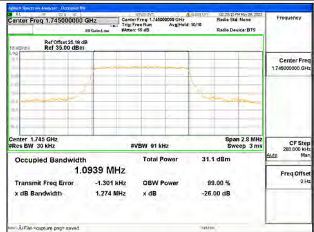
Band66 / 1.4MHz / QPSK/ Mid CH
