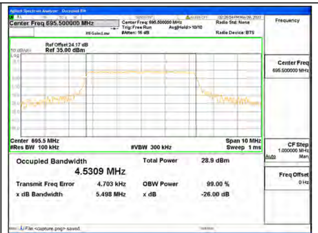
Band71 / 5MHz / 16QAM/ High CH
