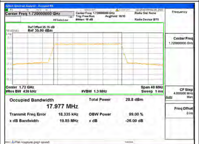
Band66 / 20MHz / 64QAM/ Low CH
