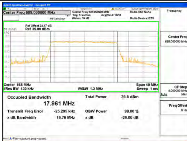
Band71 / 20MHz / 16QAM/ High CH
