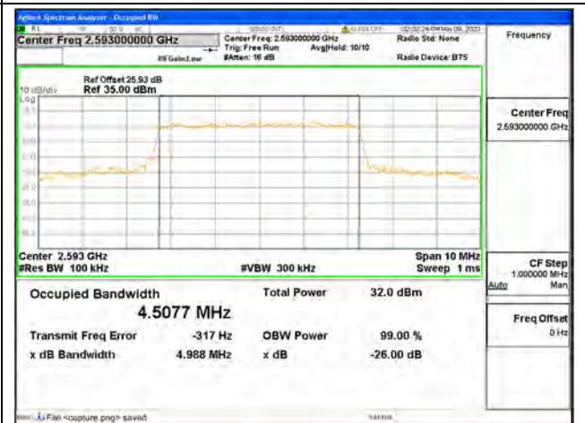
Band41 / 5MHz / 64QAM/ Mid CH
