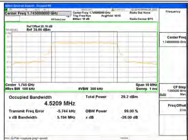
Band66 / 5MHz / 64QAM/ Mid CH
