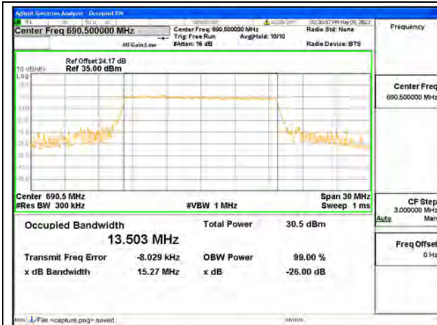
Band71 / 15MHz / QPSK/ High CH
