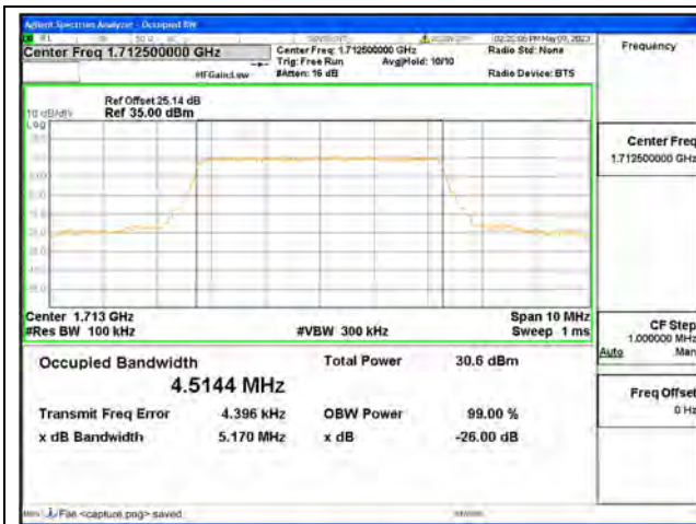
Band66 / 5MHz / QPSK/ Low CH
