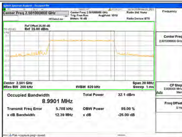
Band41 / 10MHz / 16QAM/ Low CH
