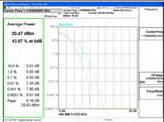
Band66 / 5MHz / Mid CH / 64QAM
