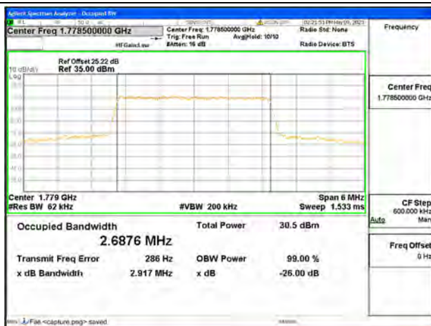
Band66 / 3MHz / 16QAM/ High CH
