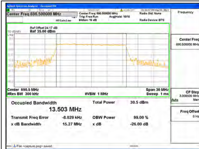
Band71 / 15MHz / QPSK/ High CH
