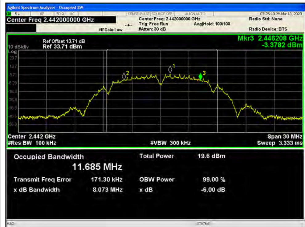
-6dB Bandwidth NVNT b 2442MHz Ant1
