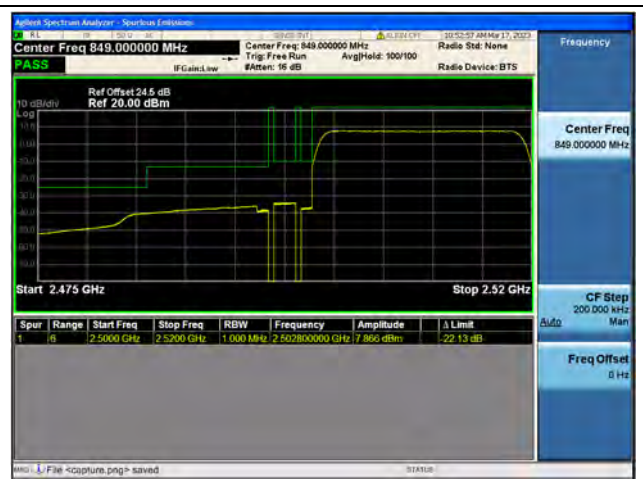
Band7 / 20MHz / Low CH / QPSK / FULL RB
