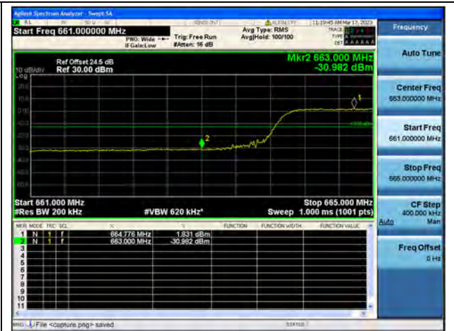
Band71 / 20MHz / Low CH / QPSK / FULL RB
