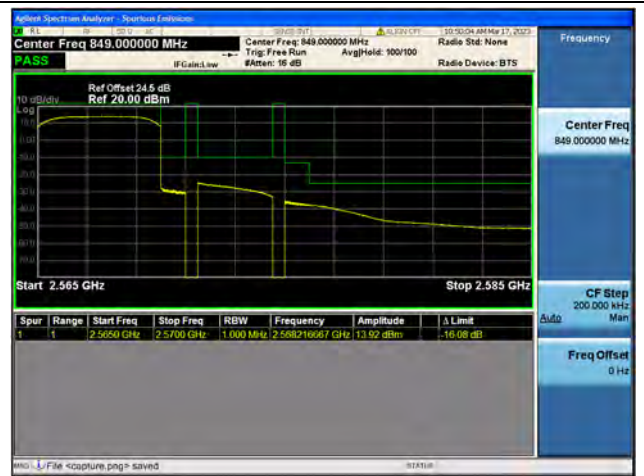
Band7 / 5MHz / High CH / QPSK / FULL RB
