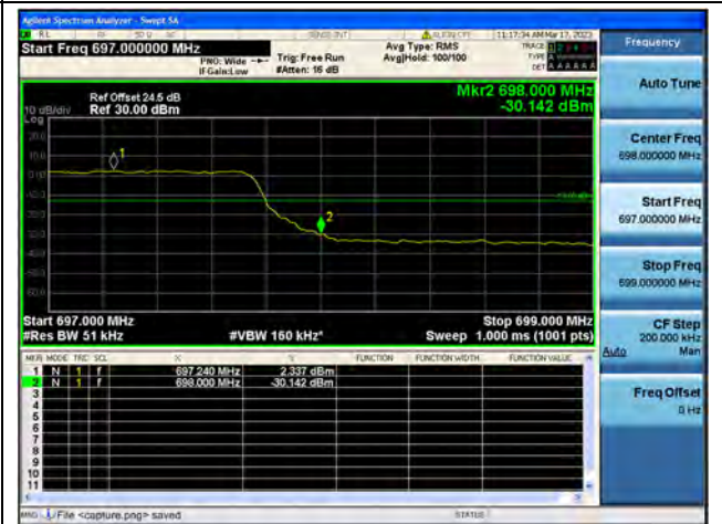
Band71 / 5MHz / High CH / QPSK / FULL RB
