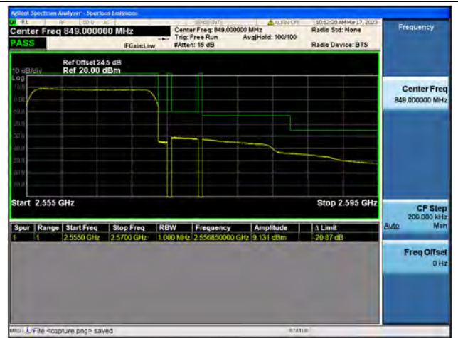
Band7 / 15MHz / High CH / QPSK / FULL RB
