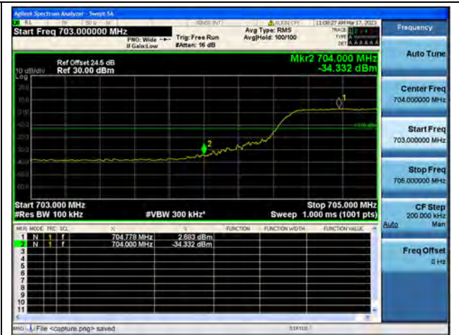
Band17 / 10MHz / Low CH / QPSK / FULL RB
