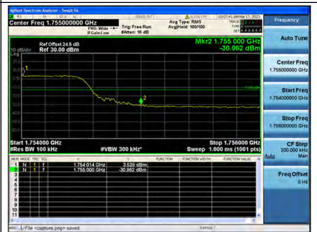
Band4 / 10MHz / High CH / QPSK / FULL RB
