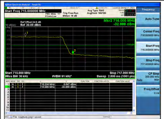
Band12 / 1.4MHz / High CH / QPSK / FULL RB
