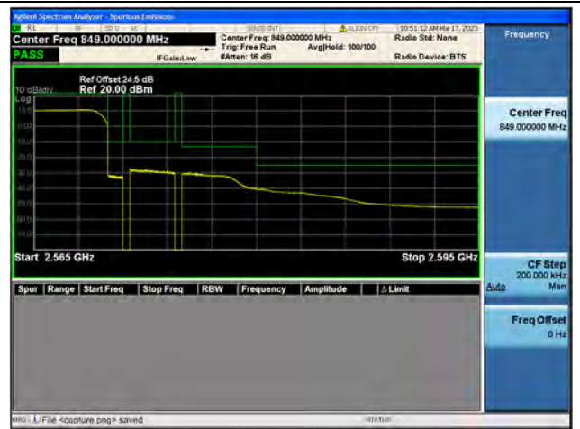
Band7 / 10MHz / High CH / QPSK / FULL RB
