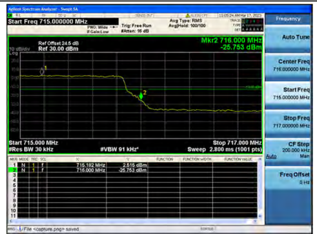
Band12 / 3MHz / High CH / QPSK / FULL RB
