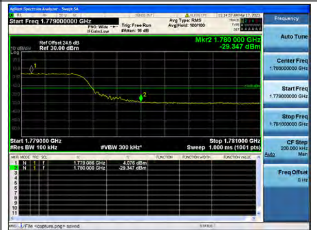
Band66 / 10MHz / High CH / QPSK / FULL RB
