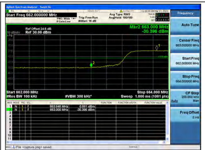
Band71 / 10MHz / Low CH / QPSK / FULL RB
