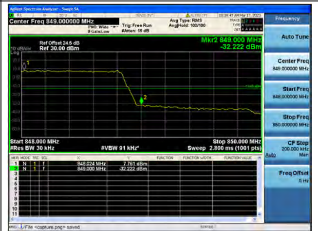
Band5 / 1.4MHz / High CH / QPSK / FULL RB
