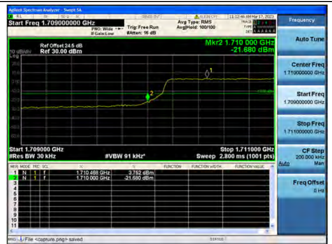
Band66 / 3MHz / Low CH / QPSK / FULL RB
