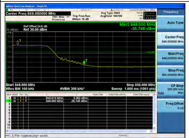
Band5 / 10MHz / High CH / QPSK / FULL RB
