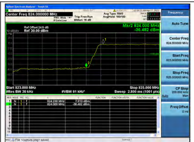
Band5 / 1.4MHz / Low CH / QPSK / FULL RB
