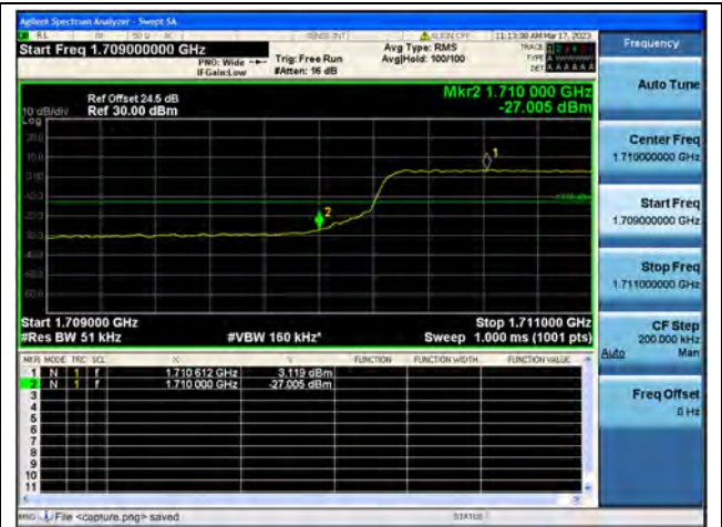
Band66 / 5MHz / Low CH / QPSK / FULL RB
