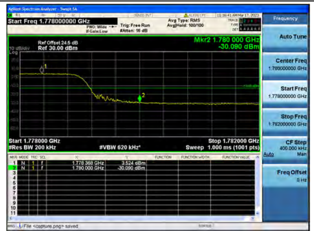
Band66 / 20MHz / High CH / QPSK / FULL RB
