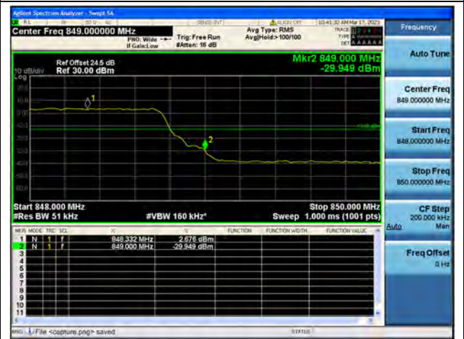
Band5 / 5MHz / High CH / QPSK / FULL RB
