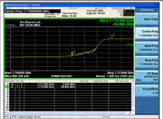
Band4 / 20MHz / Low CH / QPSK / FULL RB
