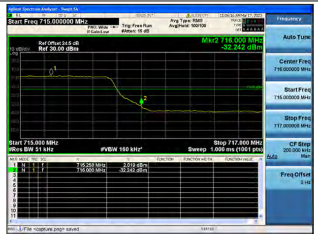
Band12 / 5MHz / High CH / QPSK / FULL RB
