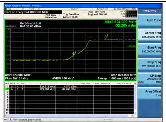
Band5 / 5MHz / Low CH / QPSK / FULL RB
