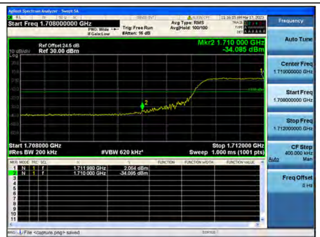
Band66 / 20MHz / Low CH / QPSK / FULL RB
