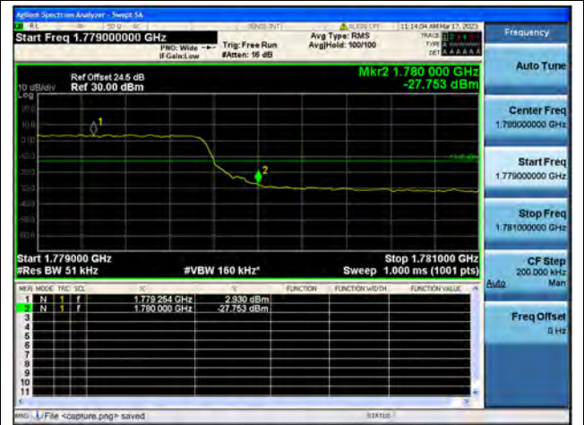
Band66 / 5MHz / High CH / QPSK / FULL RB
