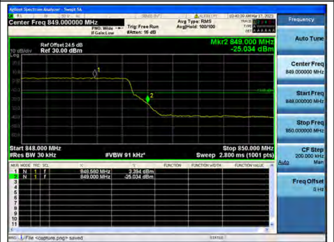
Band5 / 3MHz / High CH / QPSK / FULL RB
