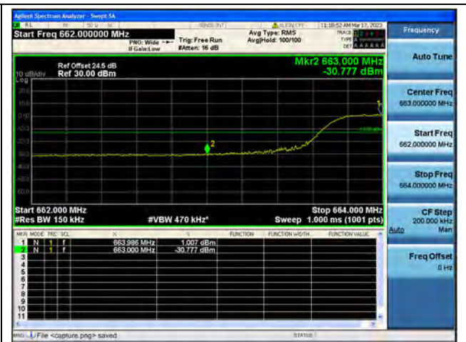
Band71 / 15MHz / Low CH / QPSK / FULL RB
