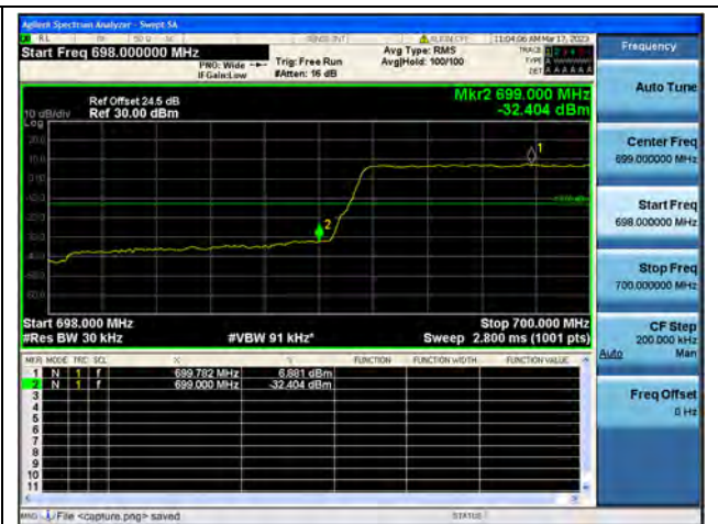
Band12 / 1.4MHz / Low CH / QPSK / FULL RB
