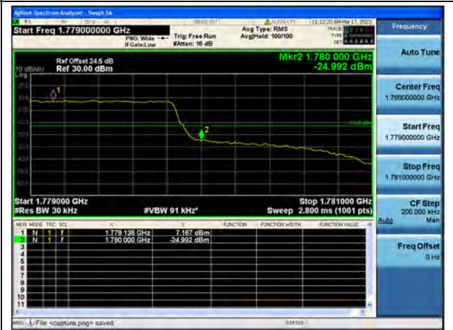
Band66 / 1.4MHz / High CH / QPSK / FULL RB
