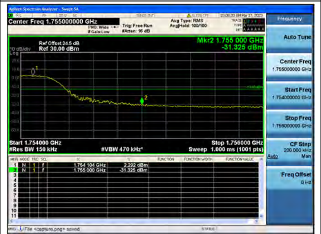
Band4 / 15MHz / High CH / QPSK / FULL RB
