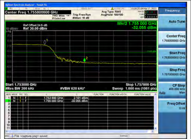
Band4 / 20MHz / High CH / QPSK / FULL RB
