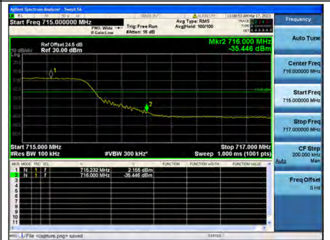
Band17 / 10MHz / High CH / QPSK / FULL RB
