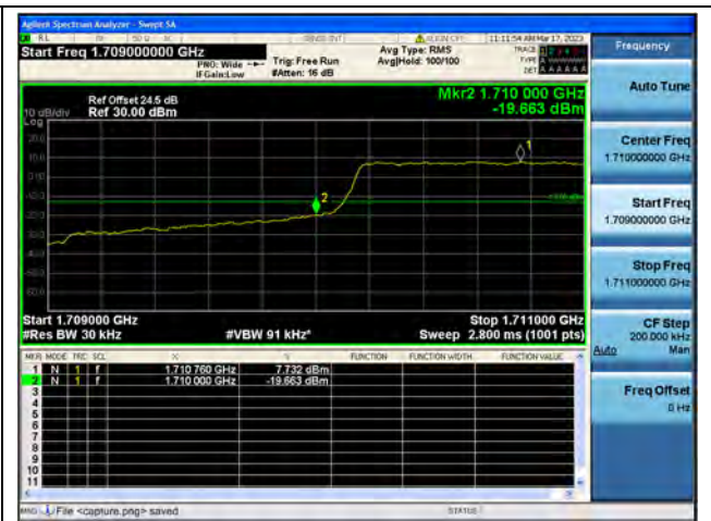
Band66 / 1.4MHz / Low CH / QPSK / FULL RB
