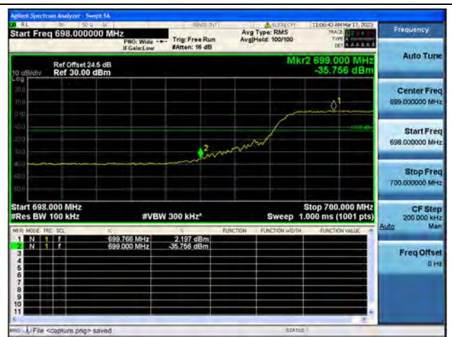
Band12 / 10MHz / Low CH / QPSK / FULL RB
