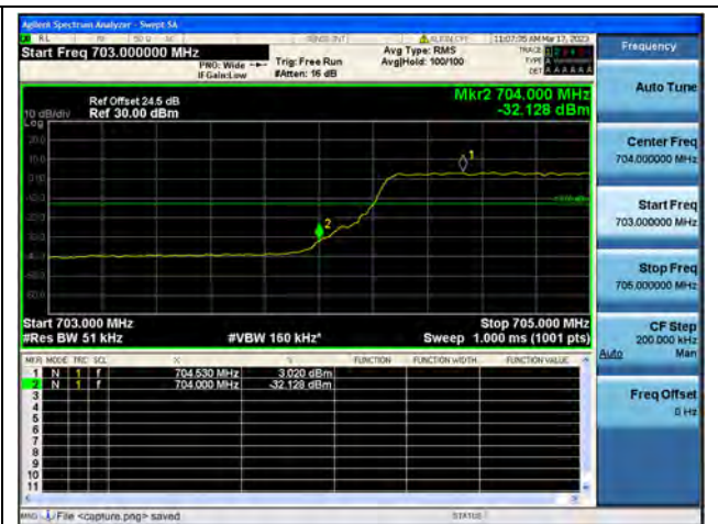
Band17 / 5MHz / Low CH / QPSK / FULL RB
