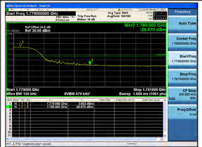
Band66 / 15MHz / High CH / QPSK / FULL RB
