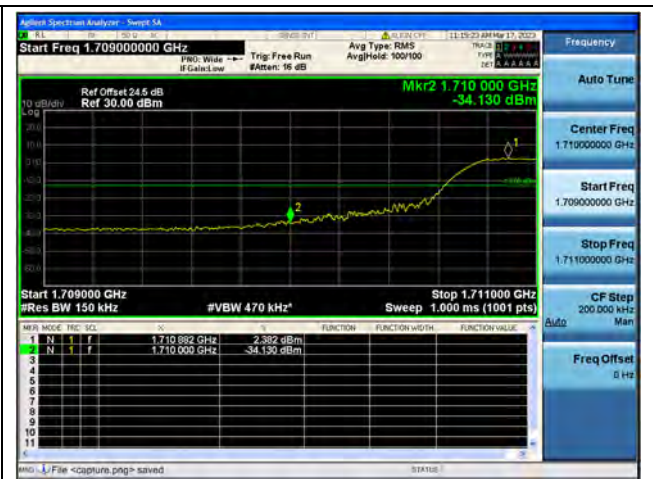
Band66 / 15MHz / Low CH / QPSK / FULL RB
