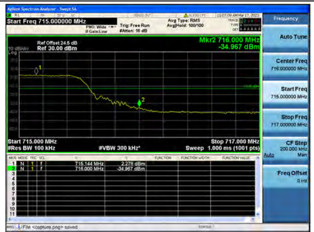
Band12 / 10MHz / High CH / QPSK / FULL RB
