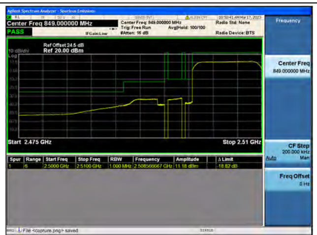
Band7 / 10MHz / Low CH / QPSK / FULL RB
