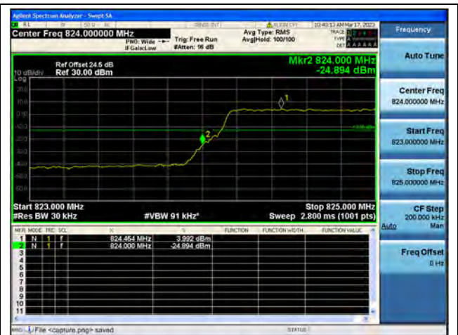
Band5 / 3MHz / Low CH / QPSK / FULL RB
