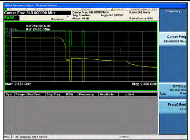
Band7 / 20MHz / High CH / QPSK / FULL RB
