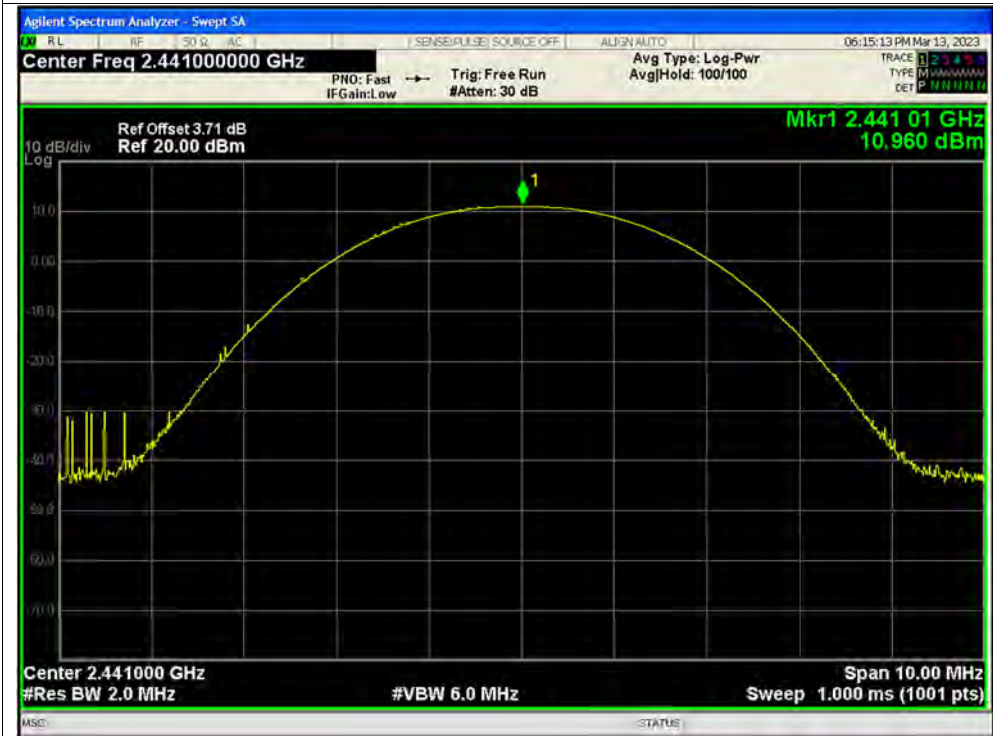
Peak Power NVNT 1-DH5 2441MHz Ant1
