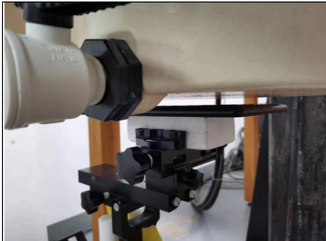
Rear Face of EUT with 0.9 cm Gap
