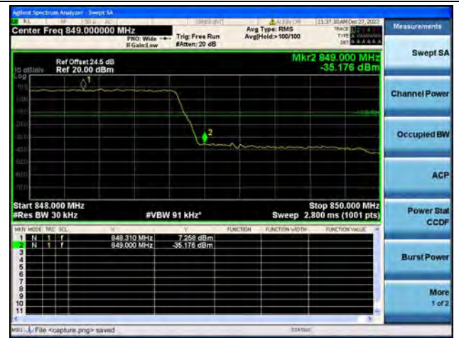
Band5 / 1.4MHz / High CH / QPSK / FULL RB
