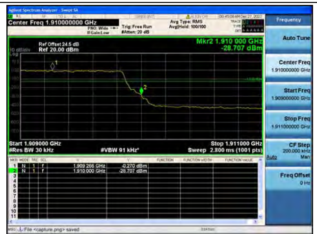
Band2 / 3MHz / High CH / QPSK / FULL RB
