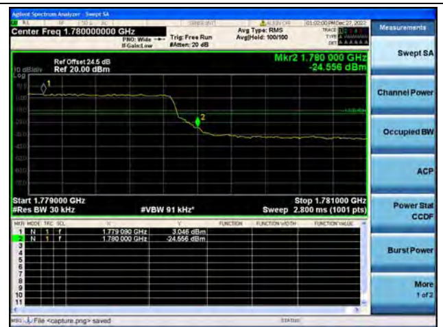
Band66 / 3MHz / High CH / QPSK / FULL RB
