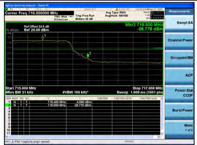
Band12 / 5MHz / High CH / QPSK / FULL RB
