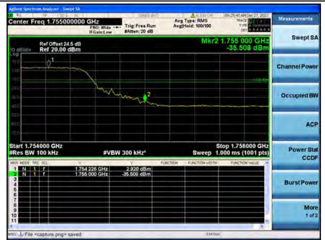
Band4 / 10MHz / High CH / QPSK / FULL RB
