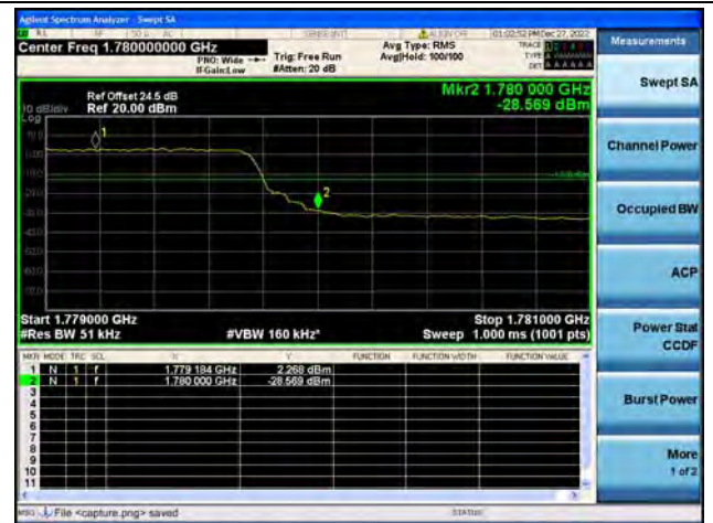
Band66 / 5MHz / High CH / QPSK / FULL RB
