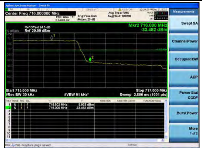
Band12 / 1.4MHz / High CH / QPSK / FULL RB
