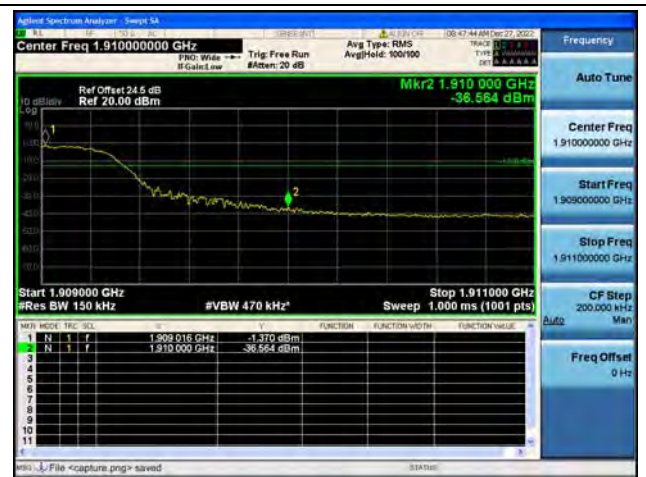
Band2 / 15MHz / High CH / QPSK / FULL RB
