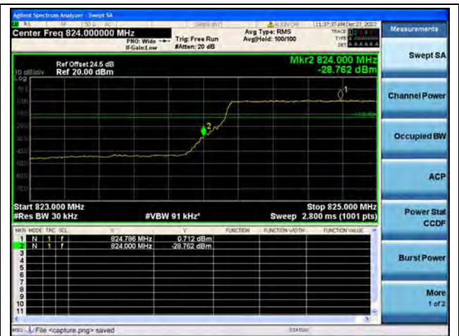
Band5 / 3MHz / Low CH / QPSK / FULL RB
