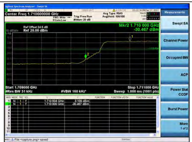
Band66 / 5MHz / Low CH / QPSK / FULL RB
