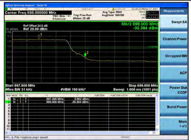
Band71 / 5MHz / High CH / QPSK / FULL RB
