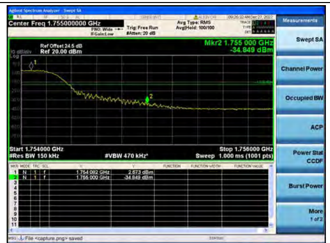
Band4 / 15MHz / High CH / QPSK / FULL RB
