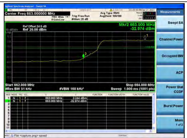
Band71 / 5MHz / Low CH / QPSK / FULL RB
