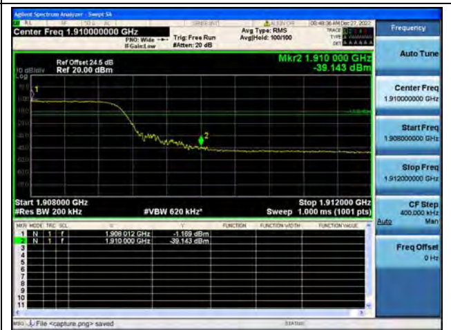
Band2 / 20MHz / High CH / QPSK / FULL RB
