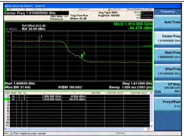
Band2 / 5MHz / High CH / QPSK / FULL RB
