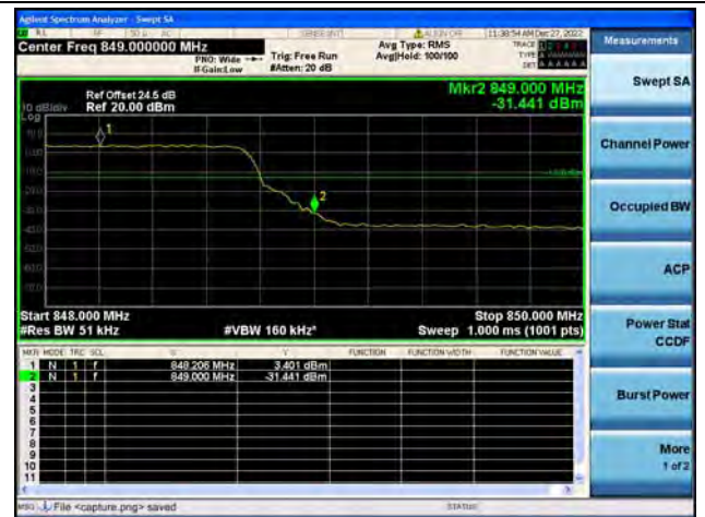
Band5 / 5MHz / High CH / QPSK / FULL RB
