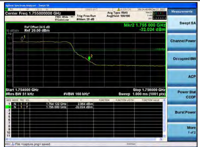
Band4 / 5MHz / High CH / QPSK / FULL RB
