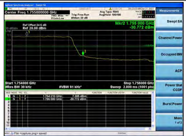
Band4 / 1.4MHz / High CH / QPSK / FULL RB
