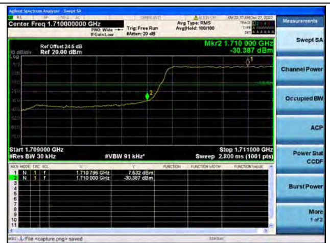
Band4 / 1.4MHz / Low CH / QPSK / FULL RB
