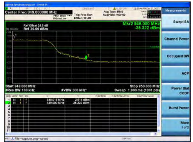
Band5 / 10MHz / High CH / QPSK / FULL RB
