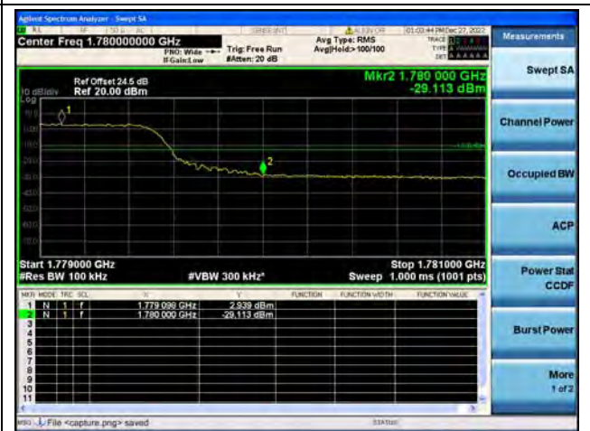
Band66 / 10MHz / High CH / QPSK / FULL RB
