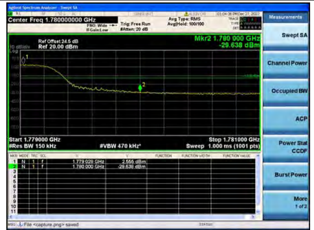
Band66 / 15MHz / High CH / QPSK / FULL RB
