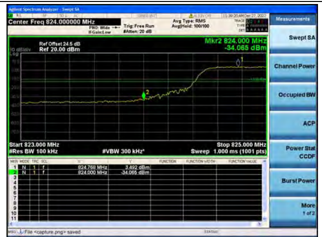
Band5 / 10MHz / Low CH / QPSK / FULL RB
