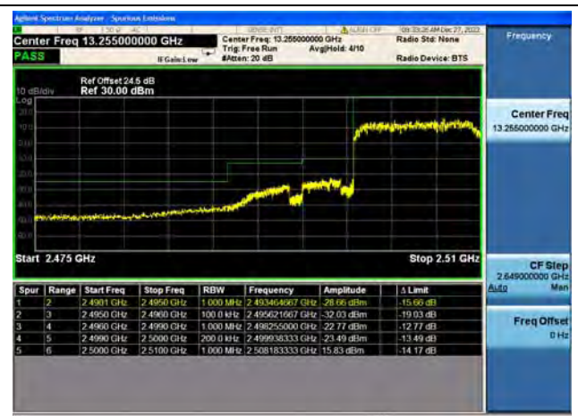
Band7 / 10MHz / Low CH / QPSK / FULL RB
