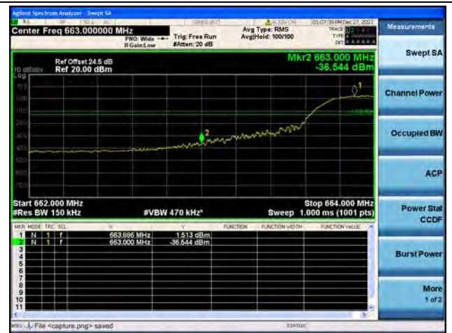
Band71 / 15MHz / Low CH / QPSK / FULL RB
