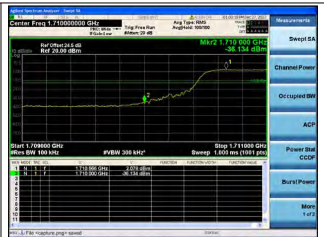
Band66 / 10MHz / Low CH / QPSK / FULL RB
