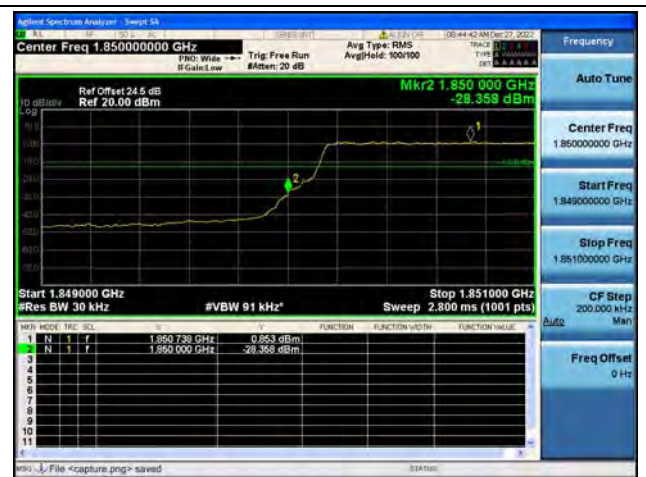
Band2 / 3MHz / Low CH / QPSK / FULL RB
