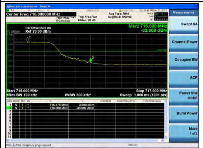
Band17 / 10MHz / High CH / QPSK / FULL RB
