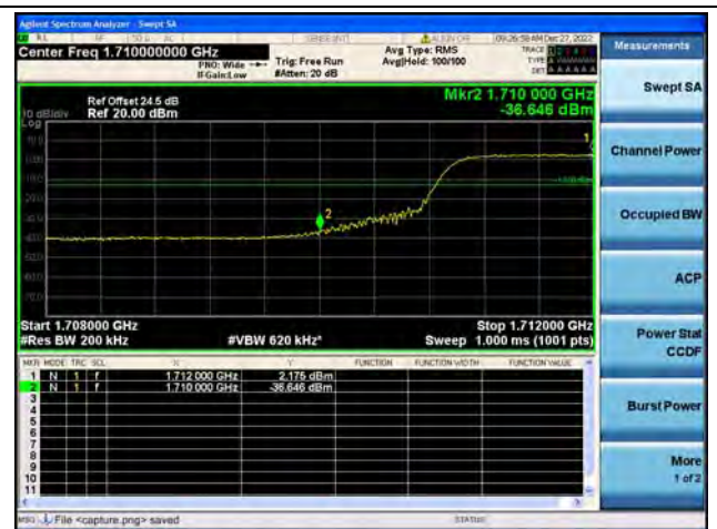
Band4 / 20MHz / Low CH / QPSK / FULL RB
