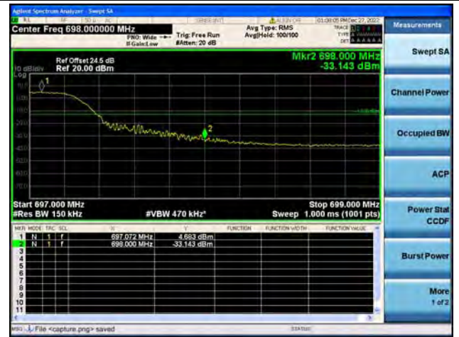
Band71 / 15MHz / High CH / QPSK / FULL RB
