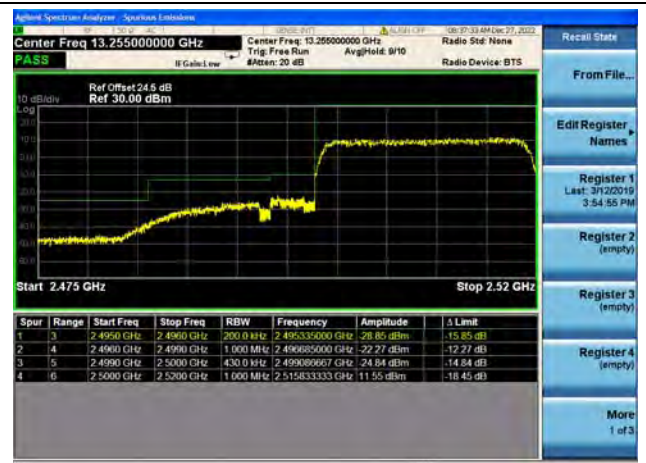
Band7 / 20MHz / Low CH / QPSK / FULL RB
