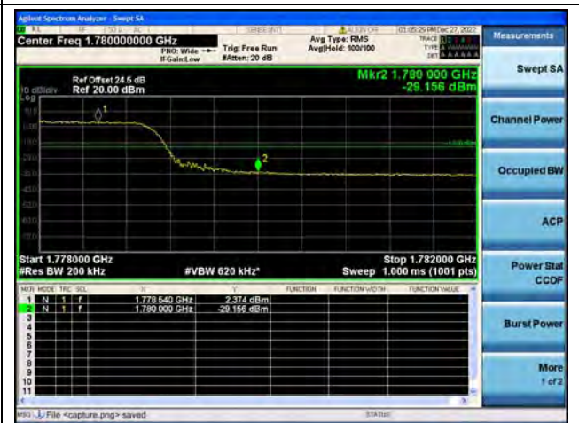
Band66 / 20MHz / High CH / QPSK / FULL RB
