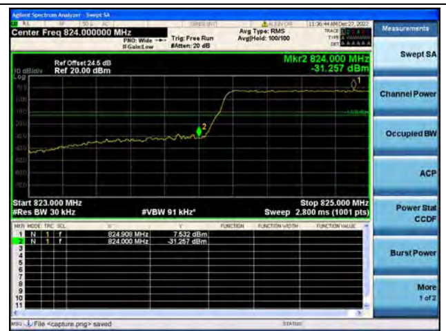
Band5 / 1.4MHz / Low CH / QPSK / FULL RB
