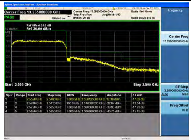
Band7 / 15MHz / High CH / QPSK / FULL RB
