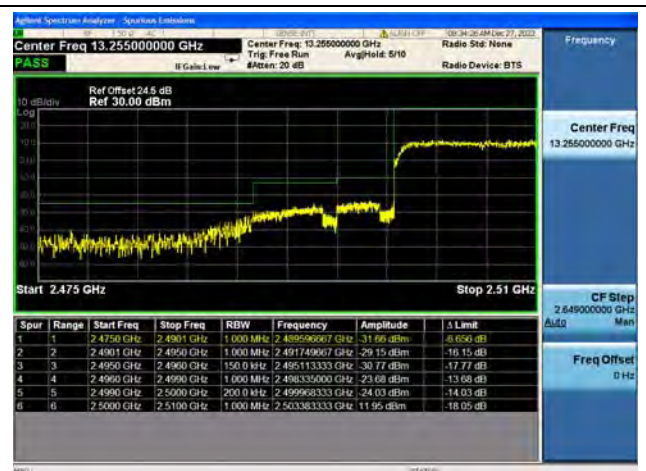
Band7 / 15MHz / Low CH / QPSK / FULL RB
