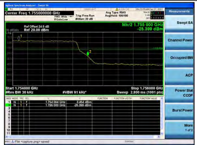
Band4 / 3MHz / High CH / QPSK / FULL RB
