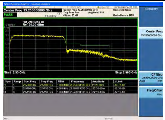
Band7 / 20MHz / High CH / QPSK / FULL RB
