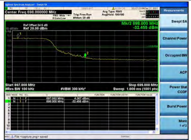
Band71 / 10MHz / High CH / QPSK / FULL RB
