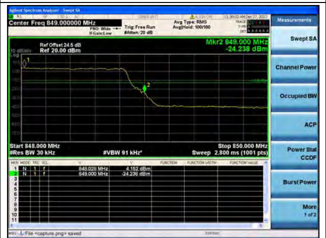
Band5 / 3MHz / High CH / QPSK / FULL RB
