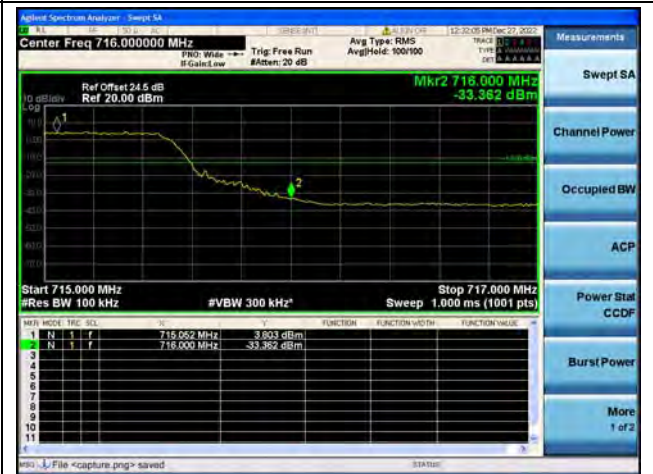
Band12 / 10MHz / High CH / QPSK / FULL RB
