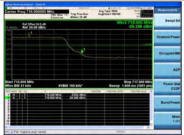
Band17 / 5MHz / High CH / QPSK / FULL RB
