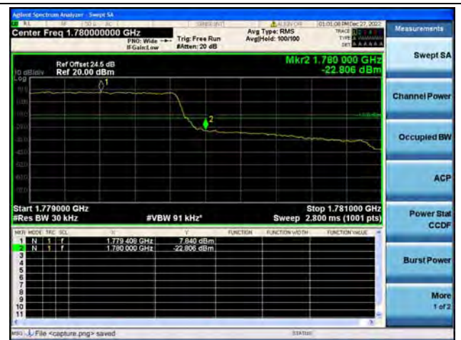
Band66 / 1.4MHz / High CH / QPSK / FULL RB
