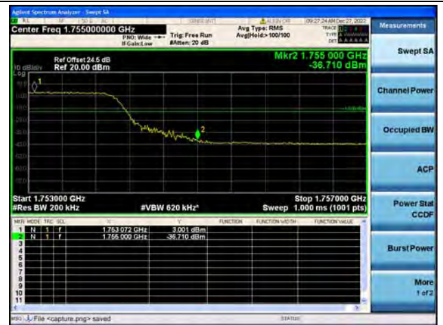
Band4 / 20MHz / High CH / QPSK / FULL RB
