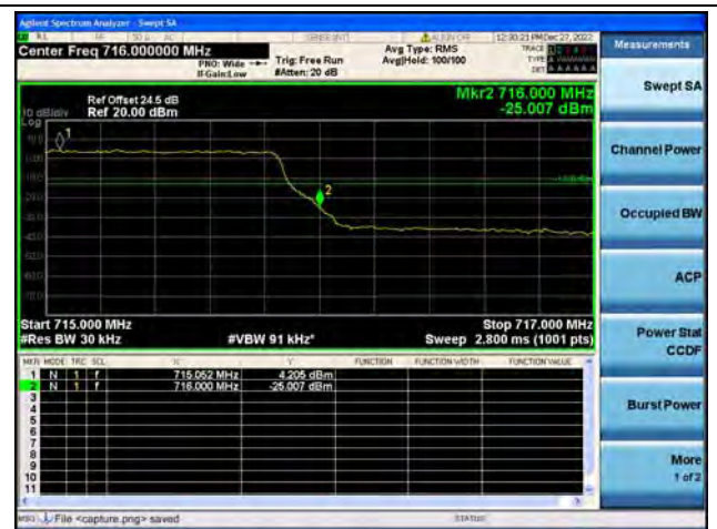
Band12 / 3MHz / High CH / QPSK / FULL RB
