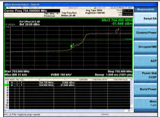
Band17 / 5MHz / Low CH / QPSK / FULL RB
