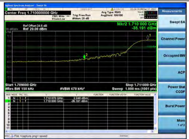
Band66 / 15MHz / Low CH / QPSK / FULL RB
