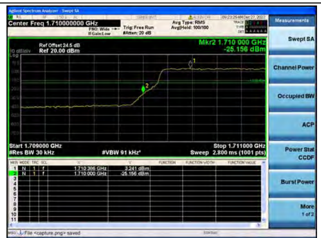
Band4 / 3MHz / Low CH / QPSK / FULL RB
