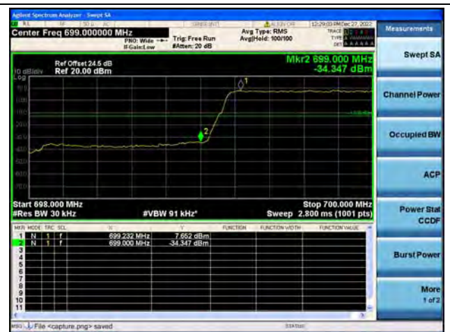
Band12 / 1.4MHz / Low CH / QPSK / FULL RB
