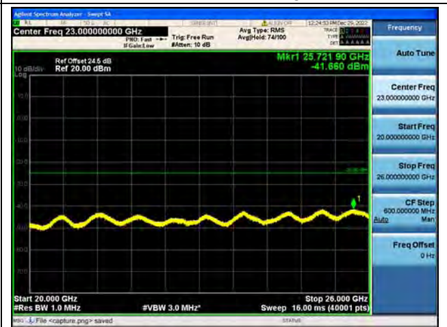
Band7-20G-26G / 10MHz / High CH / 16QAM
