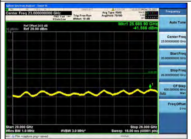
Band7-20G-26G / 5MHz / High CH / 64QAM
