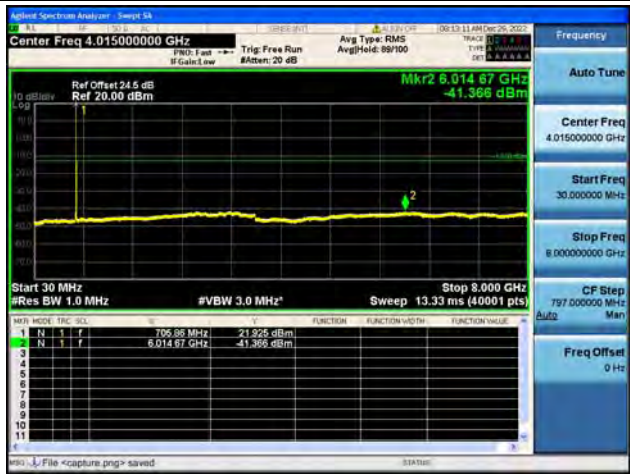
Band17 / 10MHz / Mid CH / 64QAM
