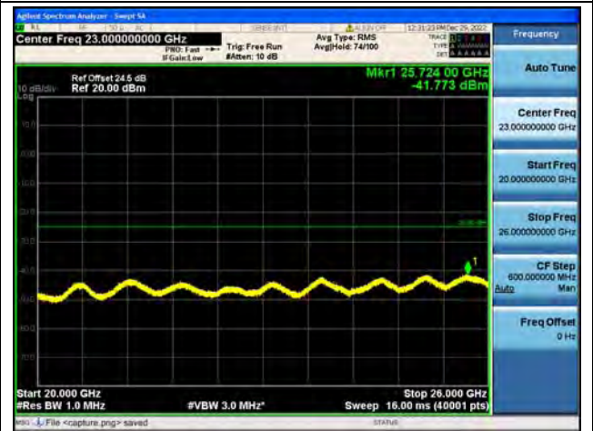
Band7-20G-26G / 20MHz / Mid CH / 16QAM
