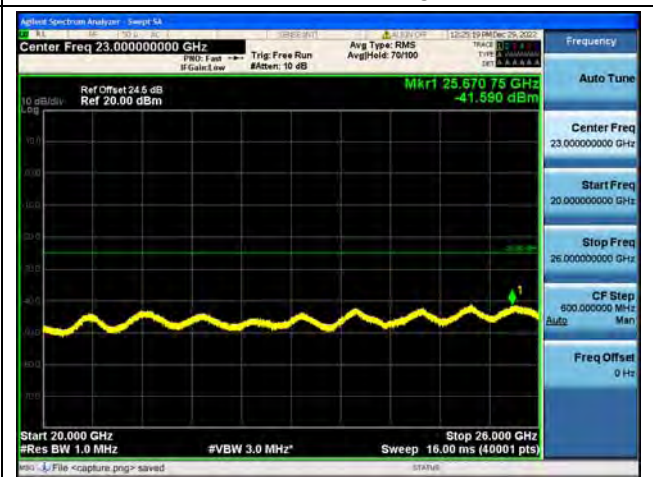
Band7-20G-26G / 10MHz / High CH / 64QAM
