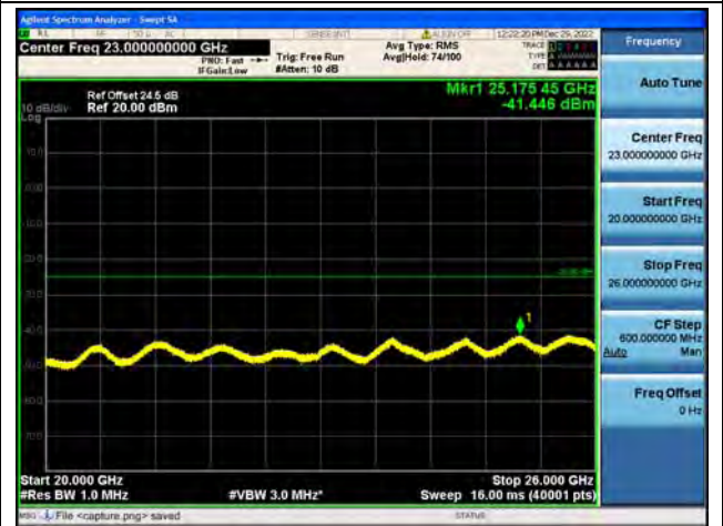
Band7-20G-26G / 10MHz / Low CH / 16QAM
