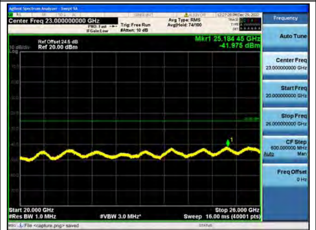
Band7-20G-26G / 15MHz / Mid CH / 16QAM
