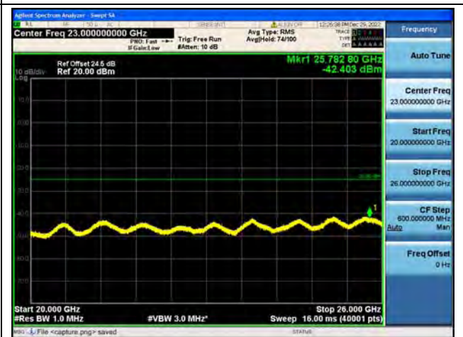
Band7-20G-26G / 15MHz / Low CH / 64QAM
