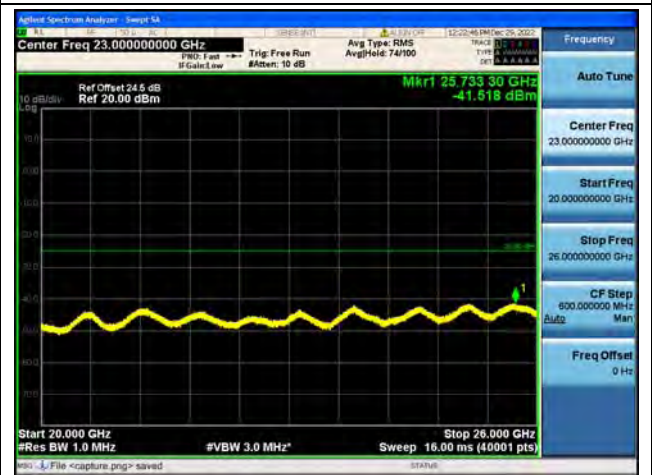
Band7-20G-26G / 10MHz / Low CH / 64QAM
