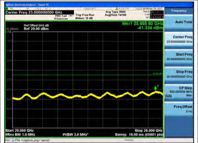
Band7-20G-26G / 10MHz / Mid CH / 16QAM
