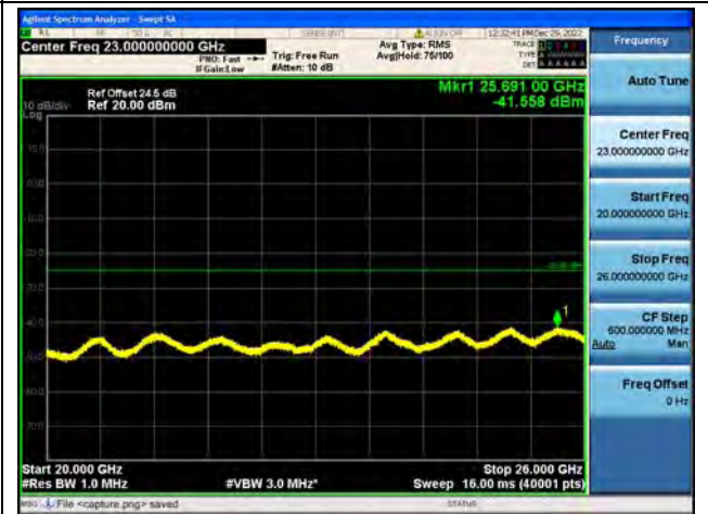
Band7-20G-26G / 20MHz / High CH / 16QAM
