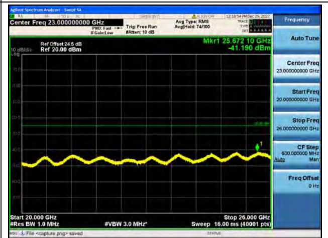
Band7-20G-26G / 5MHz / Low CH / 64QAM
