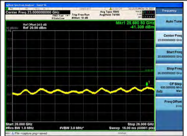
Band7-20G-26G / 5MHz / High CH / 16QAM
