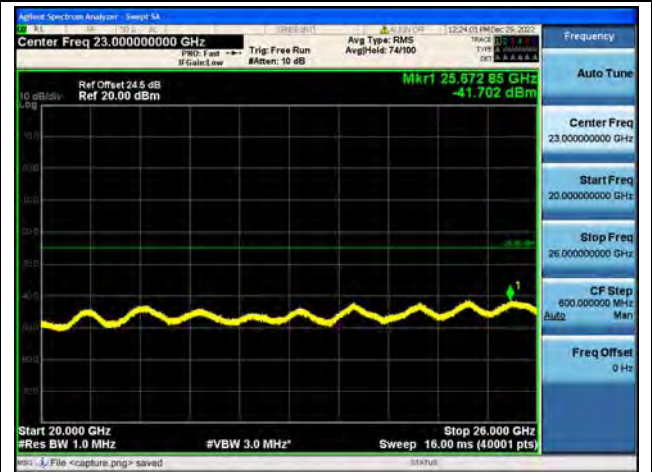
Band7-20G-26G / 10MHz / Mid CH / 64QAM
