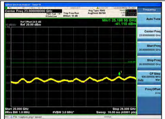
Band7-20G-26G / 15MHz / High CH / QPSK
