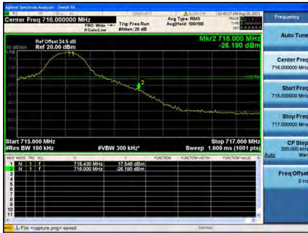
Band12 / 10MHz / High CH / QPSK / 1 RB
