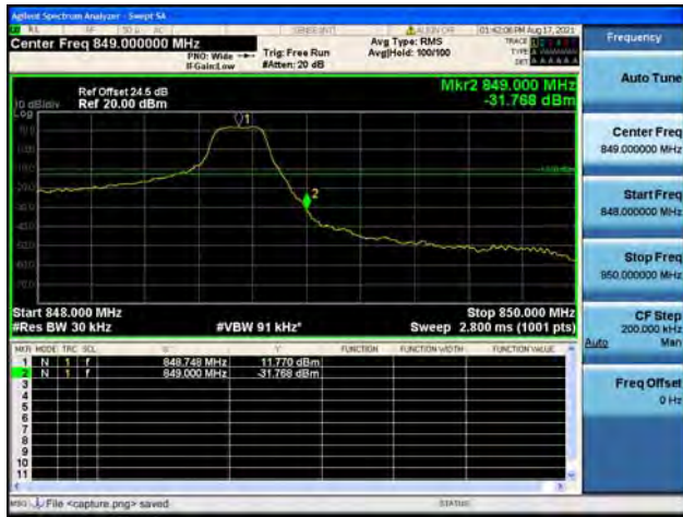
Band5 / 1.4MHz / High CH / QPSK / 1 RB
