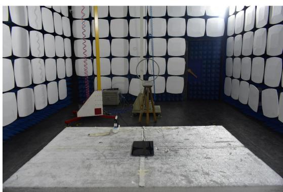
3. Radiated emission (9KHz-30MHz)
