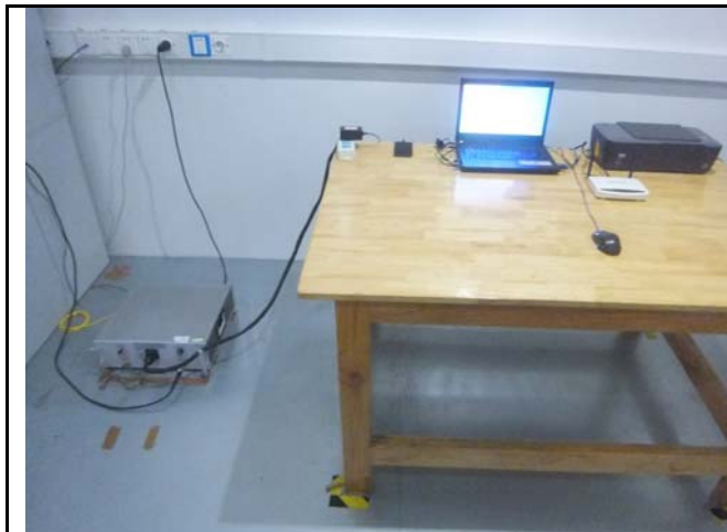
Conducted Emissions Test Setup – Front View
