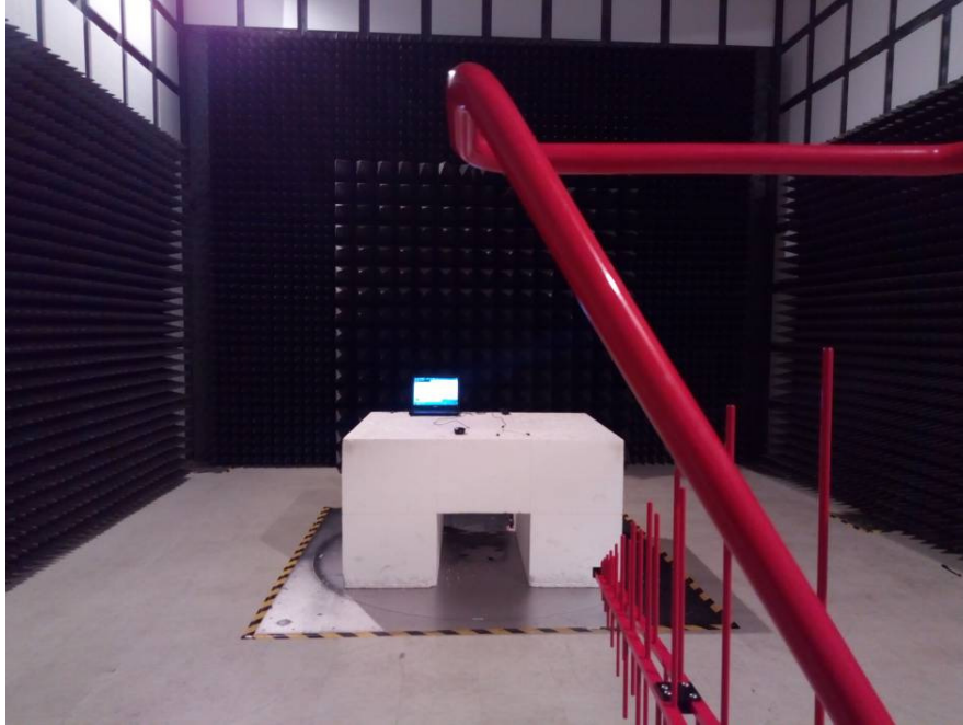
Radiated Emissions – Front View (Below 1 GHz)
