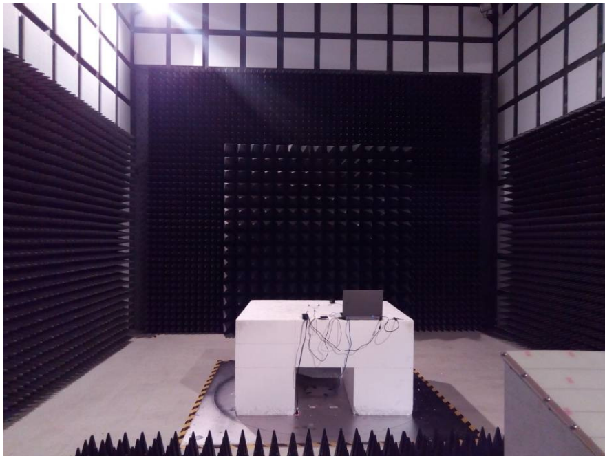
Radiated Emissions – Rear View (Above 1 GHz)
