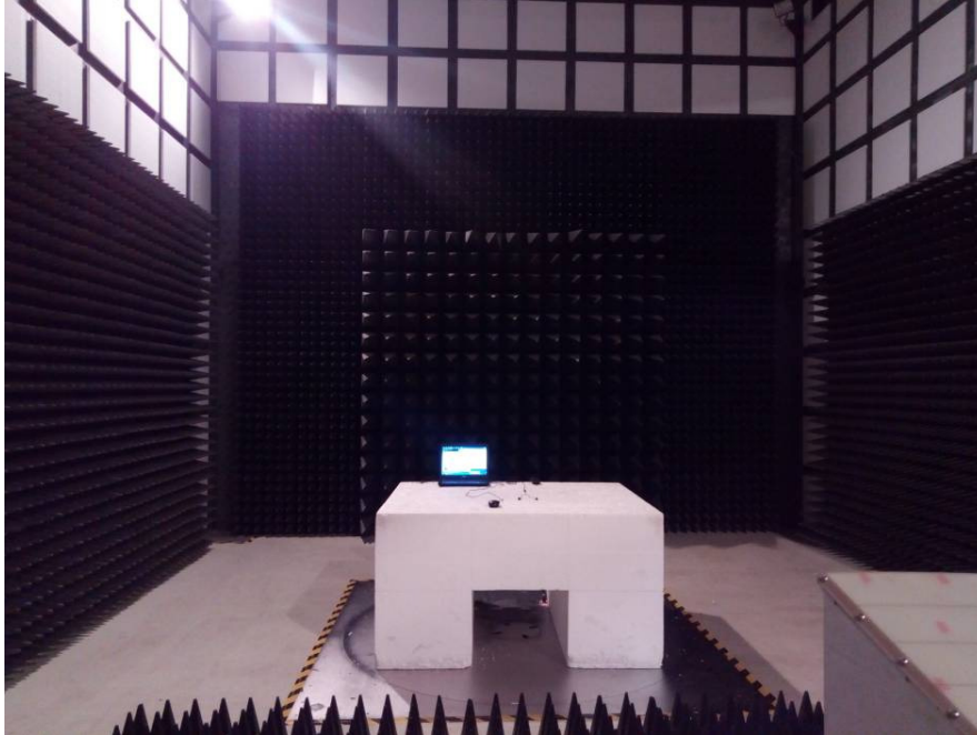
Radiated Emissions – Front View (Above 1 GHz)
