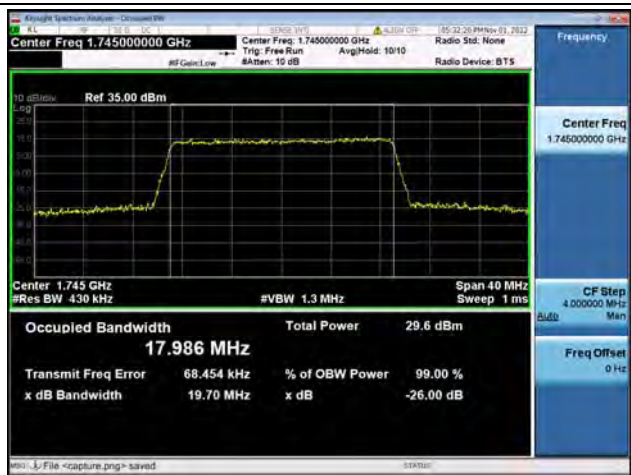
Band4 / 20MHz / QPSK/ High CH
