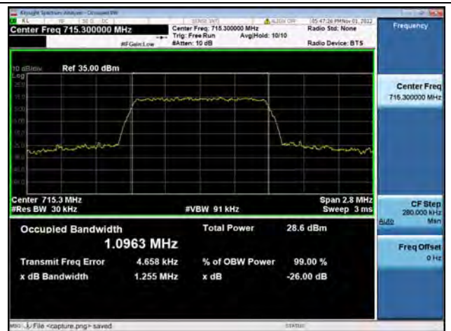
Band12 / 1.4MHz / 16QAM/ High CH
