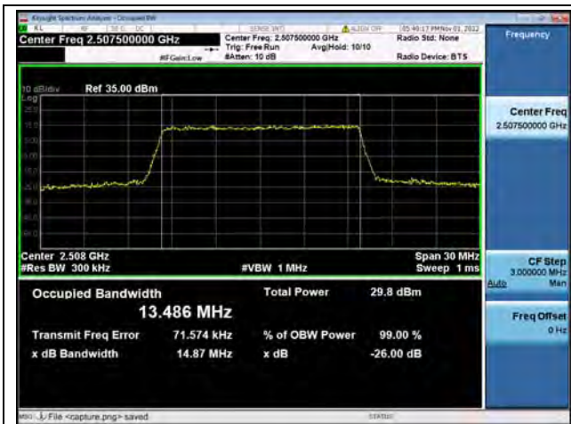
Band7 / 15MHz / QPSK/ Low CH
