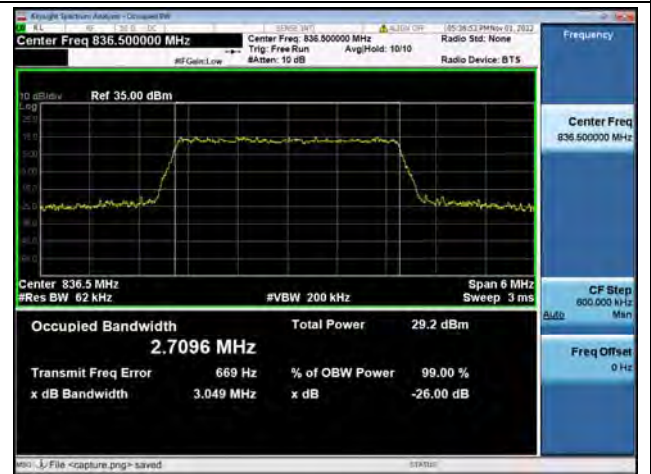
Band5 / 3MHz / 16QAM/ Mid CH
