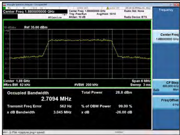
Band2 / 3MHz / QPSK/ Mid CH
