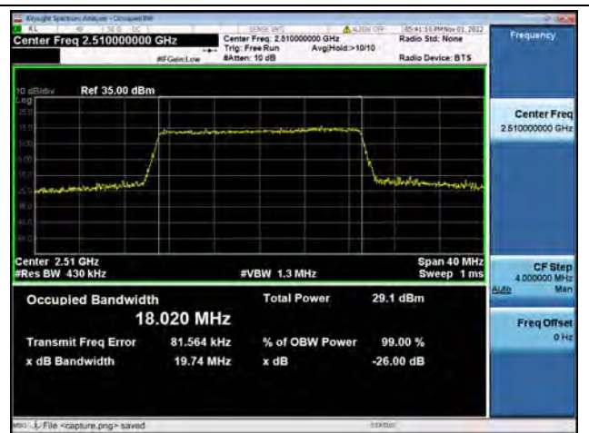
Band7 / 20MHz / 16QAM/ Low CH
