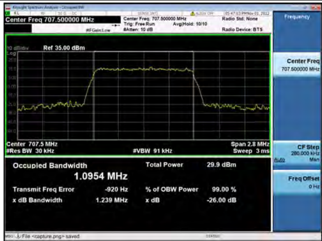
Band12 / 1.4MHz / QPSK/ Mid CH
