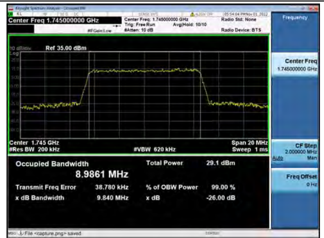
Band66 / 10MHz / 16QAM/ Mid CH
