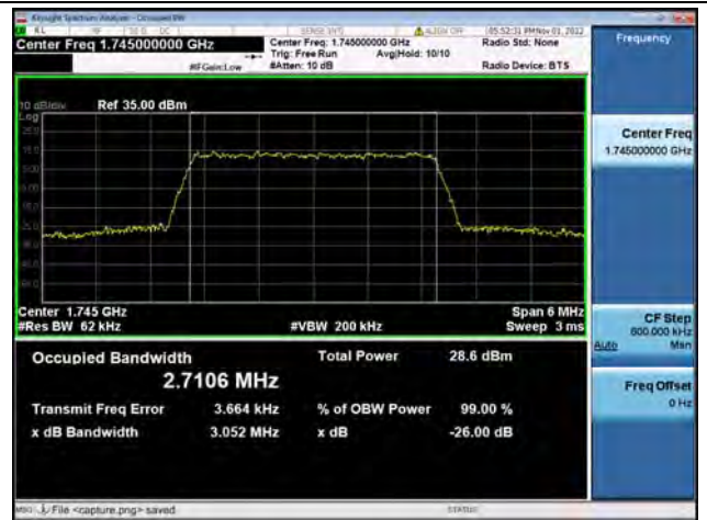
Band66 / 3MHz / 16QAM/ Mid CH
