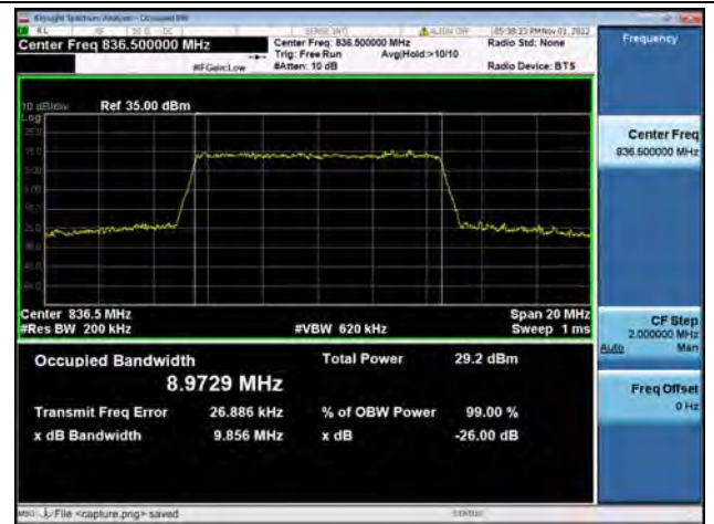
Band5 / 10MHz / 16QAM/ Mid CH
