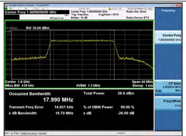
Band2 / 20MHz / 16QAM/ High CH
