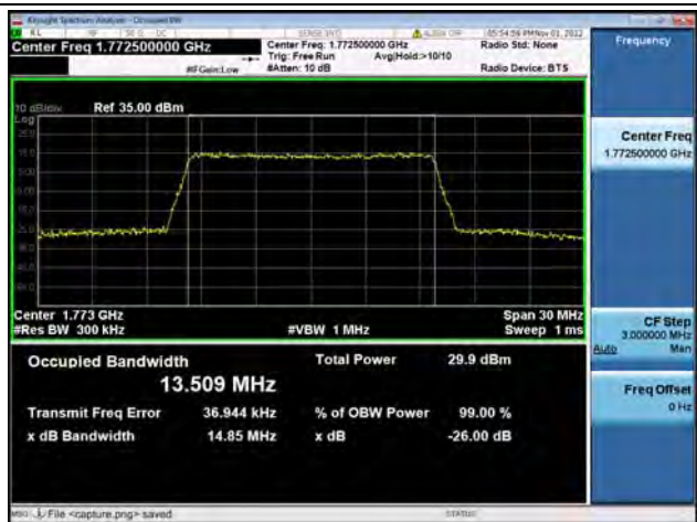
Band66 / 15MHz / QPSK/ High CH
