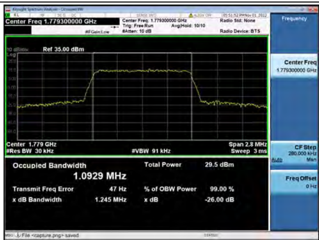
Band66 / 1.4MHz / QPSK/ High CH
