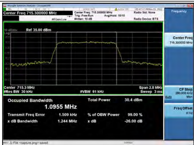
Band12 / 1.4MHz / QPSK/ High CH
