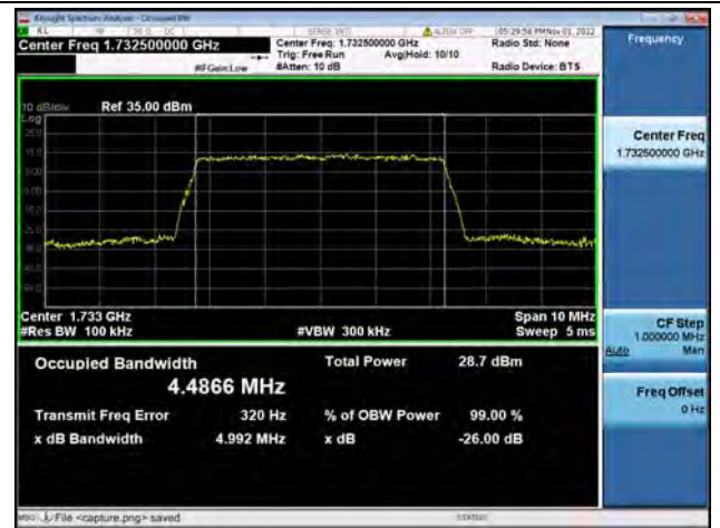
Band4 / 5MHz / 16QAM/ Mid CH
