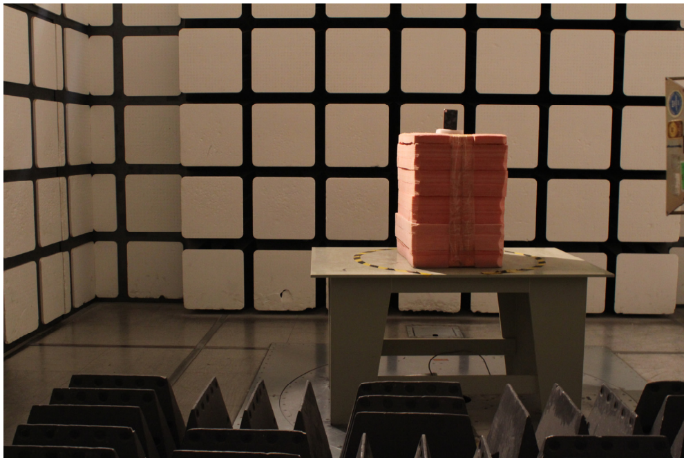
Radiated Emissions View (Above 1 GHz)
