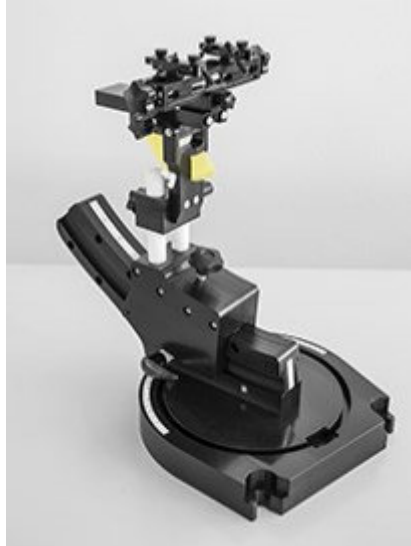
Mounting Device for Hand-Held Transmitters
