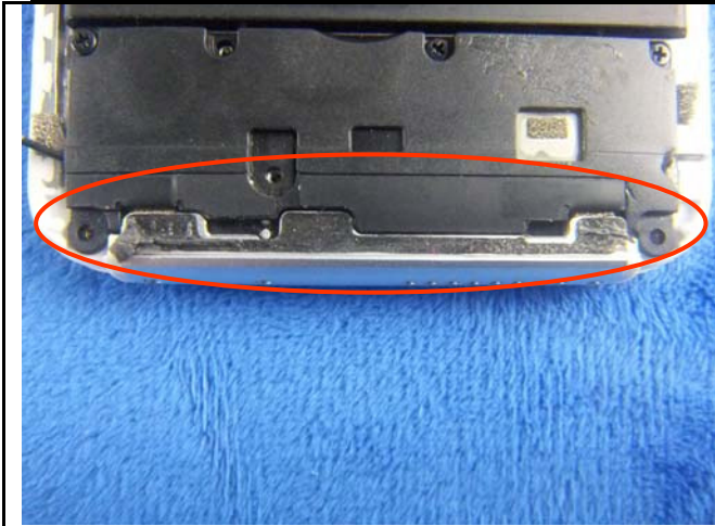
GSM/PCS/UMTS-FDD Antenna View
