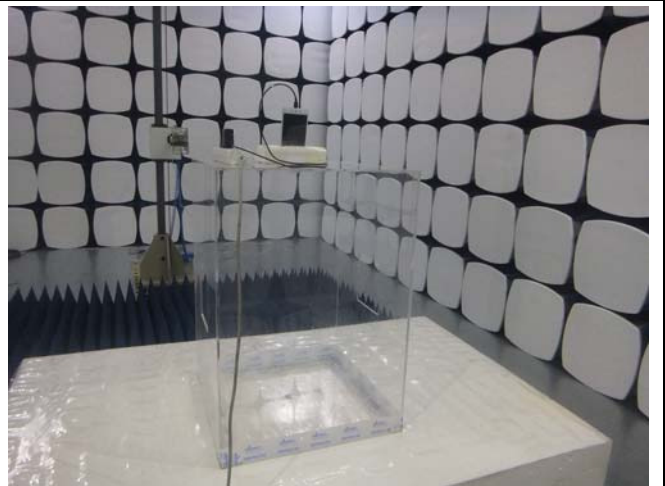
Radiated Spurious Emissions Test Setup Above 1GHz
