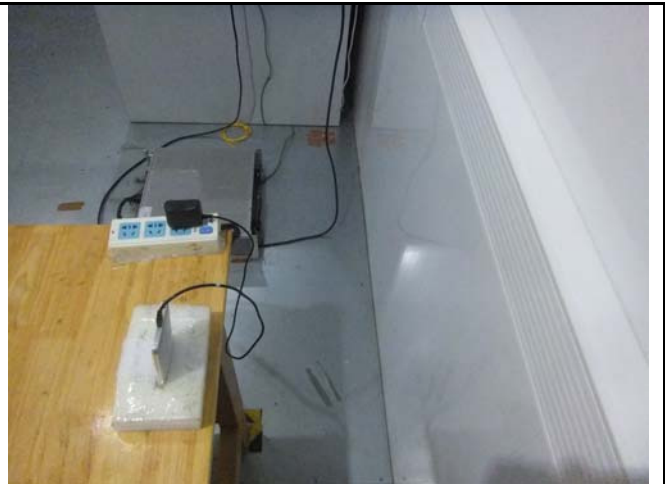
Conducted Emissions Test Setup Side View
