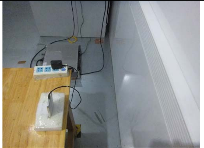
Conducted Emissions Test Setup Side View
