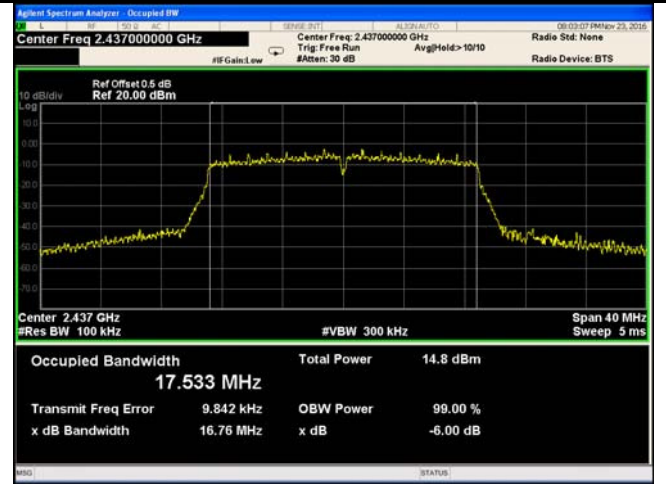
802.11n20 6dB Bandwidth - Mid CH 2437
