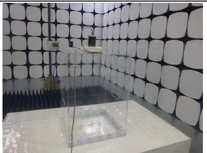
Radiated Spurious Emissions Test Setup Above 1GHz
