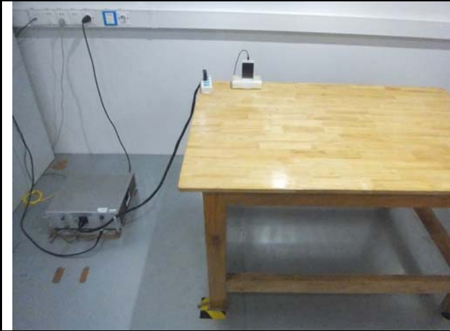
Conducted Emissions Test Setup Front View
