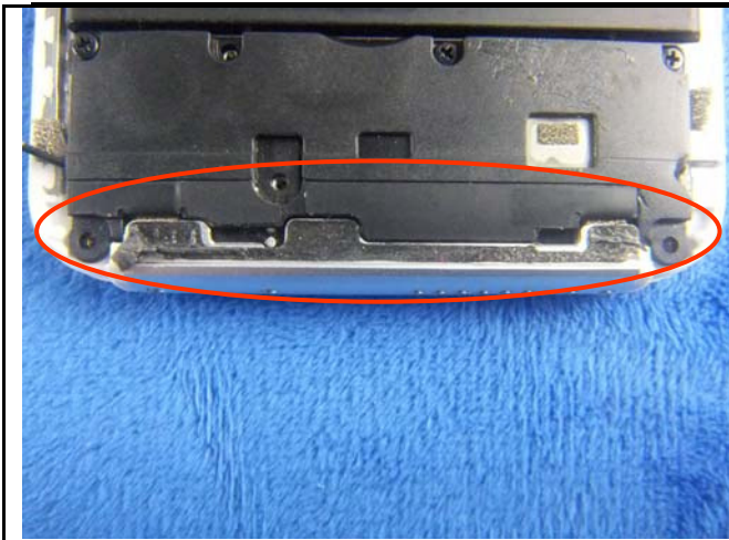
GSM/PCS/UMTS-FDD Antenna View
