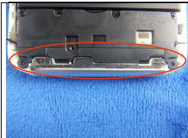
GSM/PCS/UMTS-FDD Antenna View
