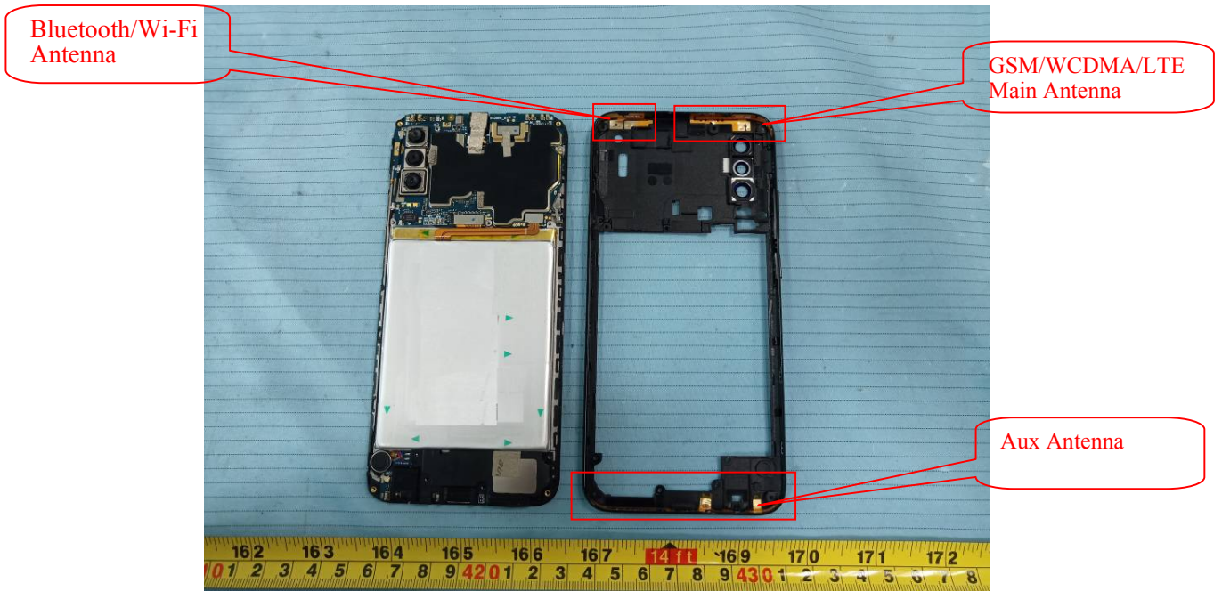
EUT – Cover off View 2
