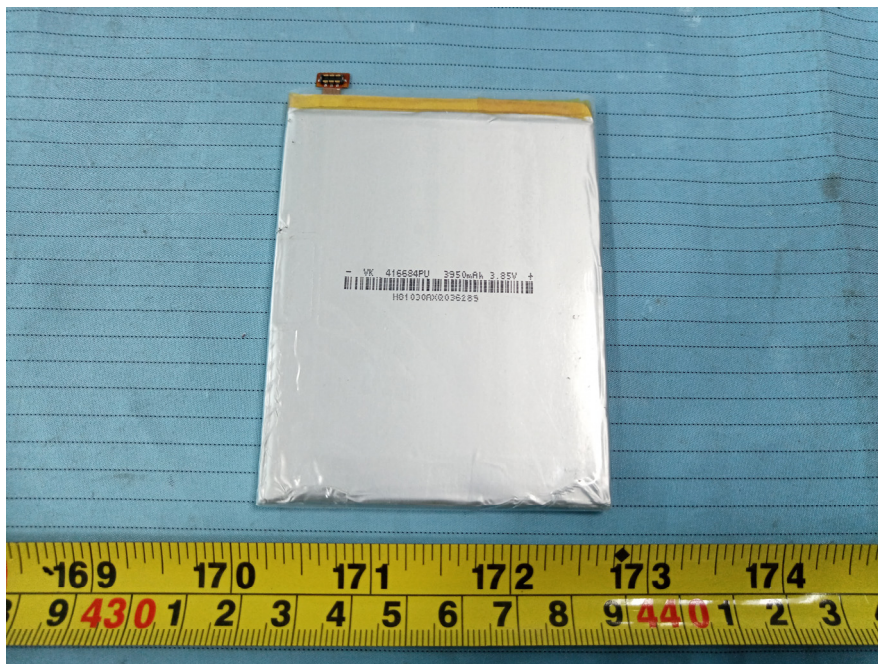
EUT – Battery View
