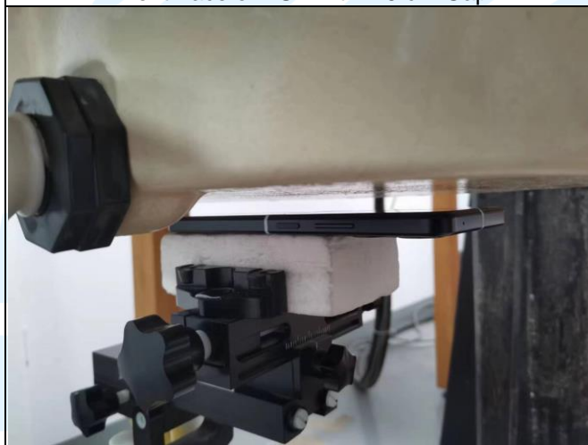
Front Face of EUT with 1.0 cm Gap
