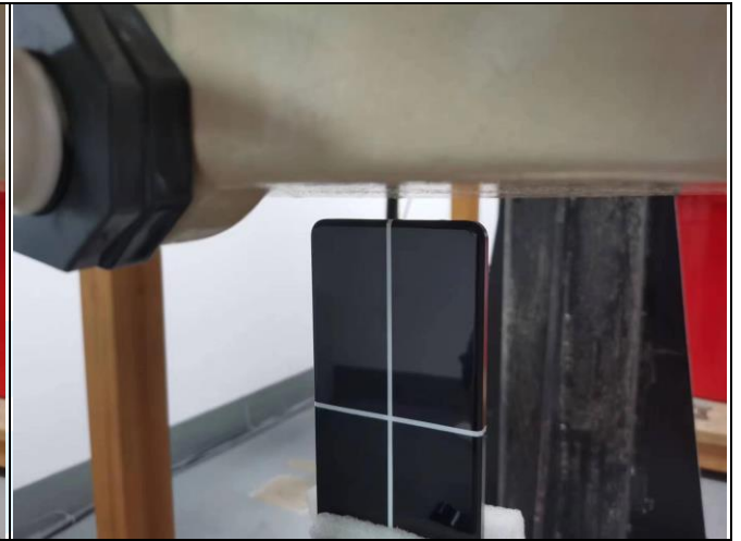
Bottom Side of EUT with 1.0 cm Gap
