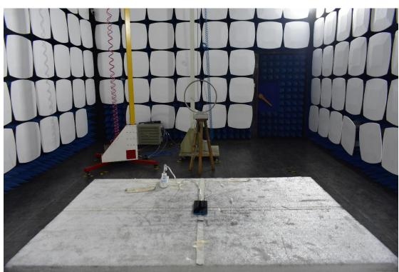
3. Radiated emission (9KHz-30MHz)
