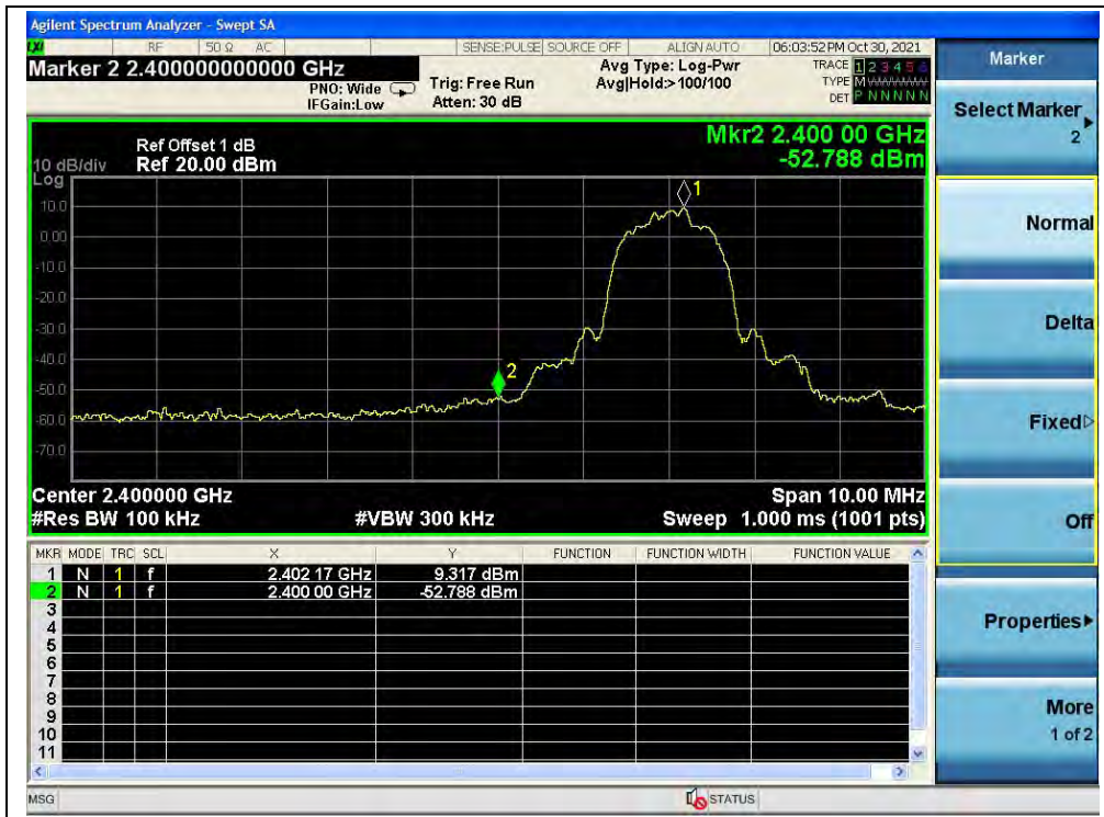
(Band edge, Channel 0, 8-DPSK)
