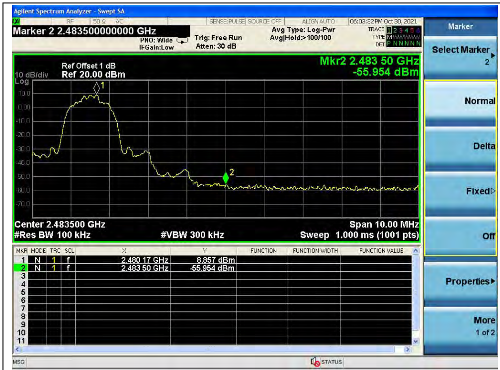
(Band edge, Channel 78, 8-DPSK)
