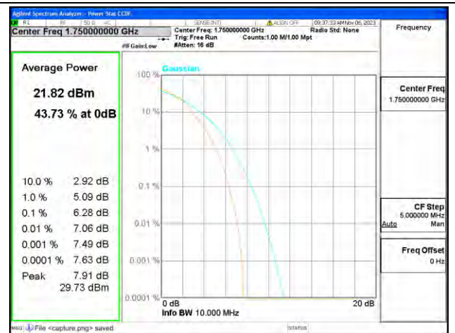
B4 / 10MHz / High CH / 16QAM
