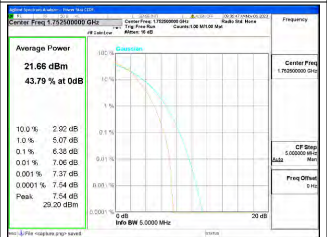
B4 / 5MHz / High CH / 16QAM
