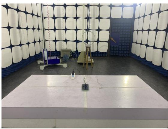
3. Radiated emission (9KHz-30MHz)
