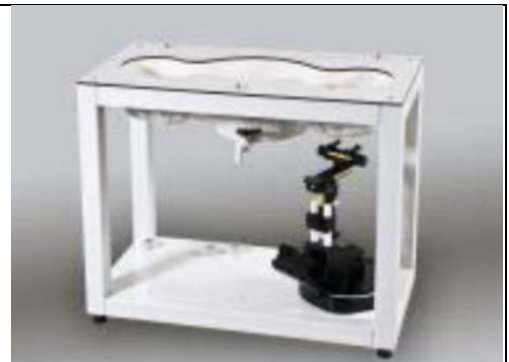
Fig. 6.8 Photo of SAM Phantom
