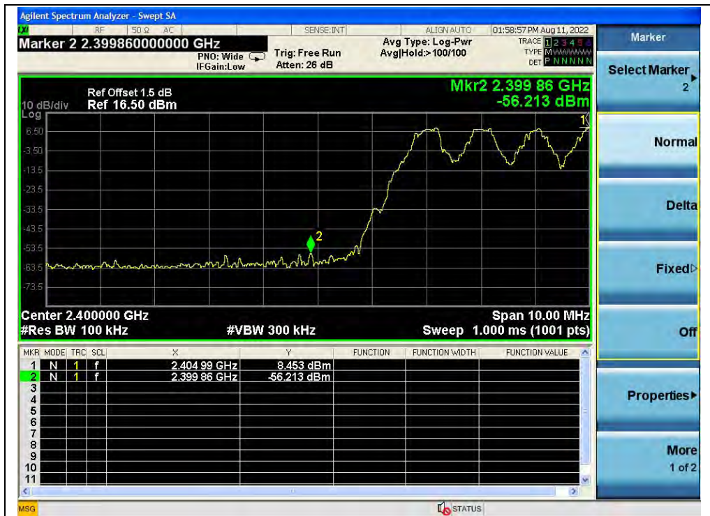
(Band edge with hopping on, Channel 0, GFSK)
