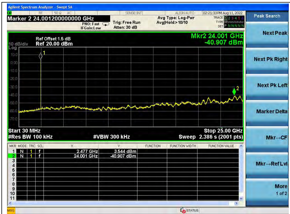
(30MHz to 25GHz, Channel 78, 8-DPSK)
