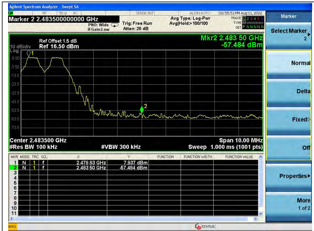
(Band edge with hopping on, Channel 78, GFSK)
