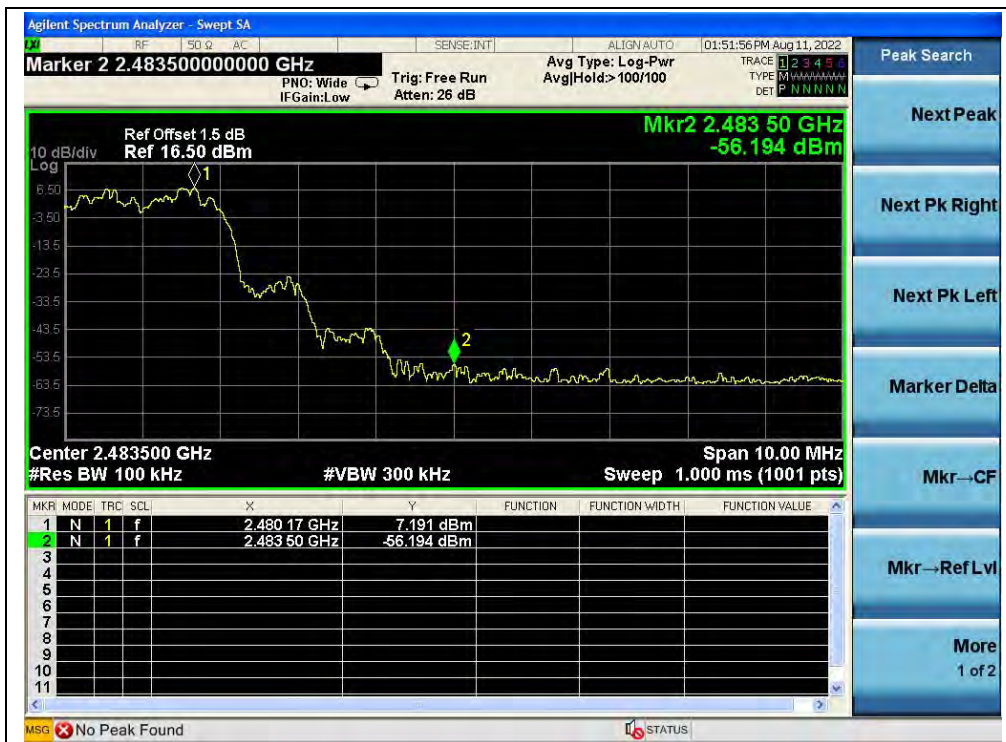
(Band edge with hopping on, Channel 78, 8-DPSK)
