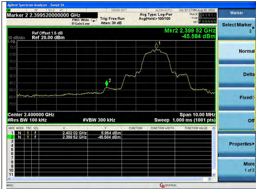
(Band edge, Channel 0, \pi/4 -DQPSK)
