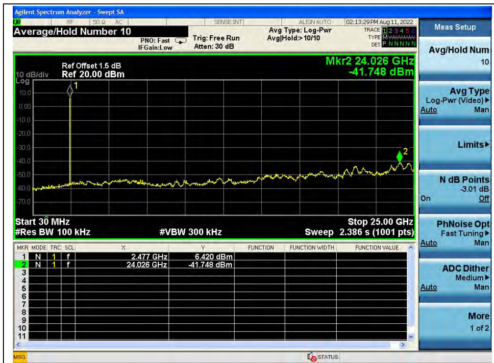
(30MHz to 25GHz, Channel 78, GFSK)
