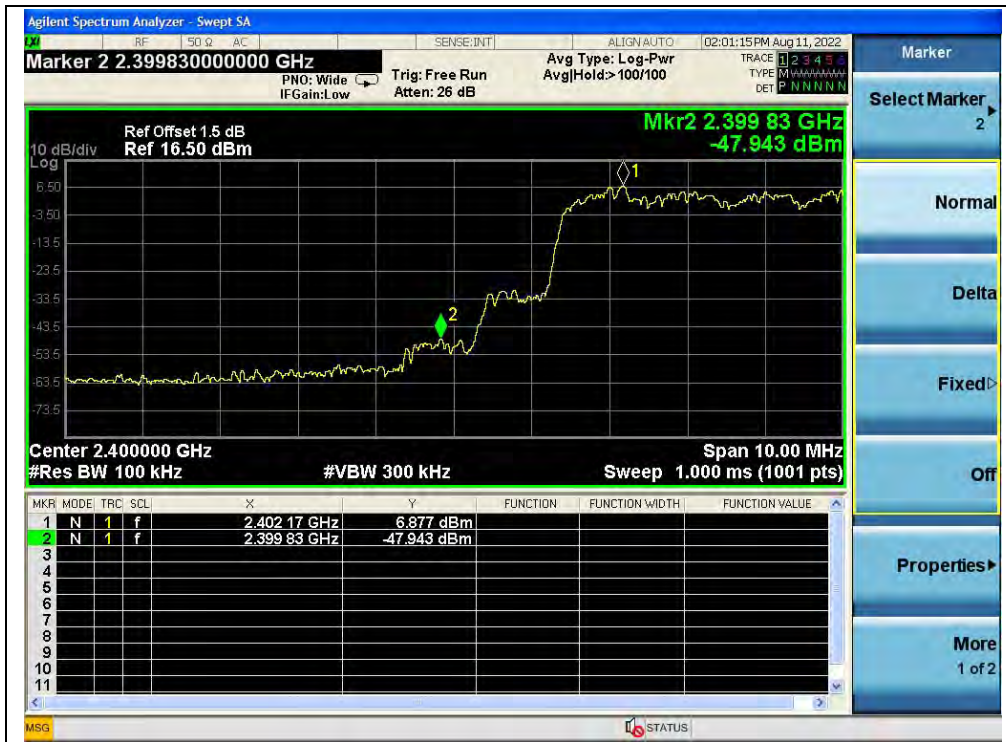
(Band edge with hopping on, Channel 0, 8-DPSK)
