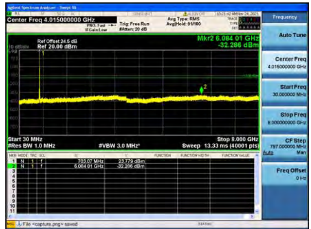
Band12 / 10MHz / High CH / QPSK
