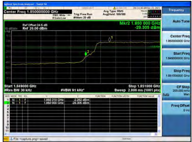
Band2 / 3MHz / High CH / QPSK / FULL RB
