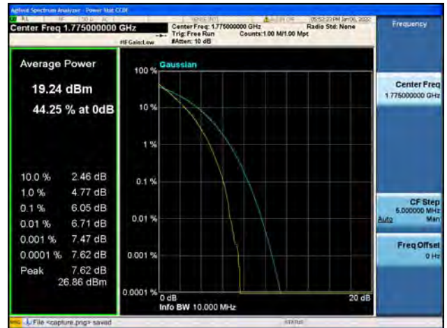
Band66 / 10MHz / High CH / 64QAM
