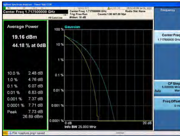
Band66 / 15MHz / Low CH / 64QAM
