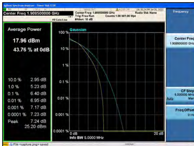
Band2 / 3MHz / High CH / 16QAM
