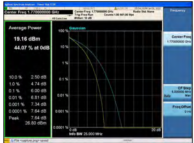
Band66 / 20MHz / High CH / 64QAM
