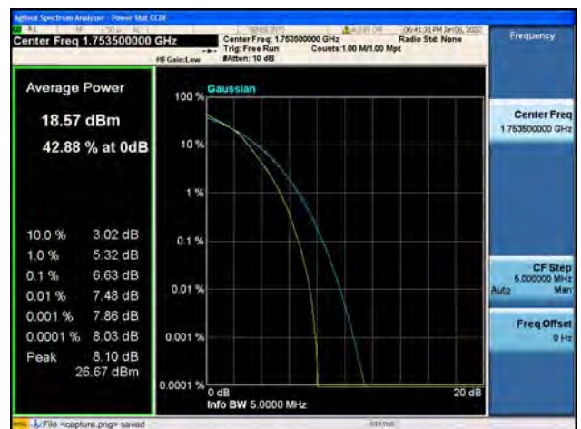
Band4 / 3MHz / High CH / 64QAM
