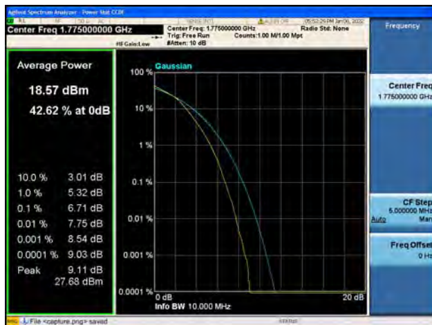
Band66 / 10MHz / High CH / 16QAM
