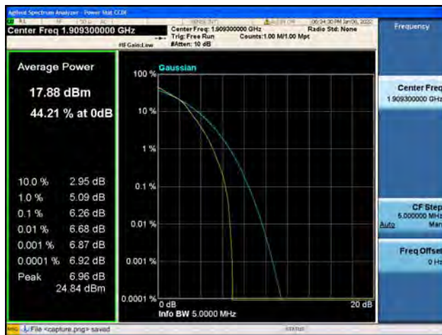
Band2 / 3MHz / Low CH / 16QAM
