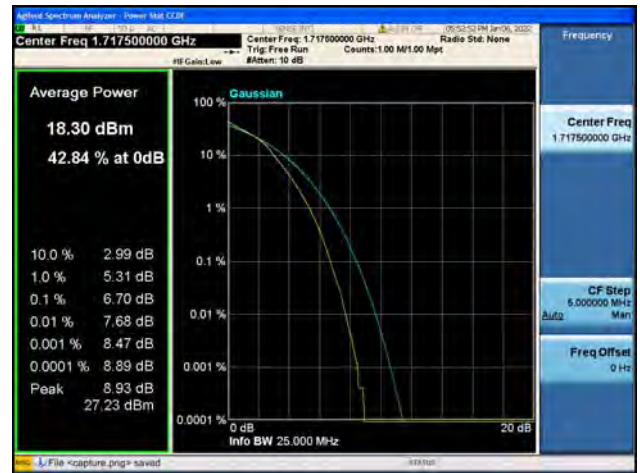
Band66 / 15MHz / Mid CH / QPSK
