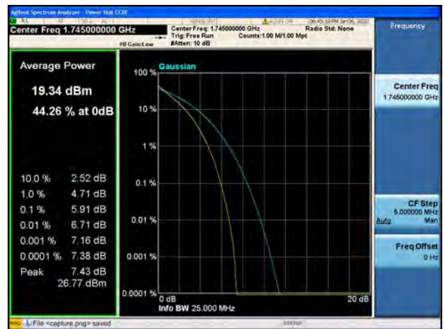
Band4 / 20MHz / High CH / 64QAM
