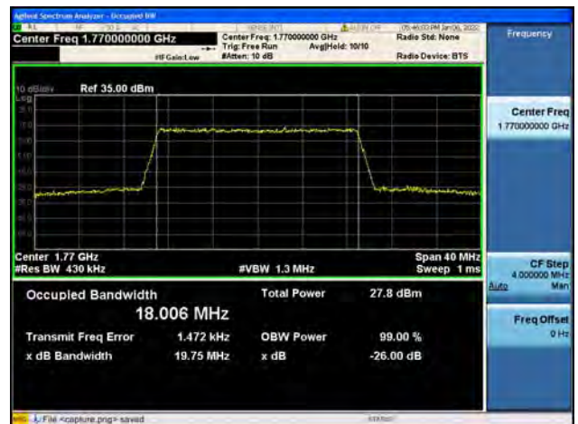
Band66 / 20MHz / High CH / 64QAM
