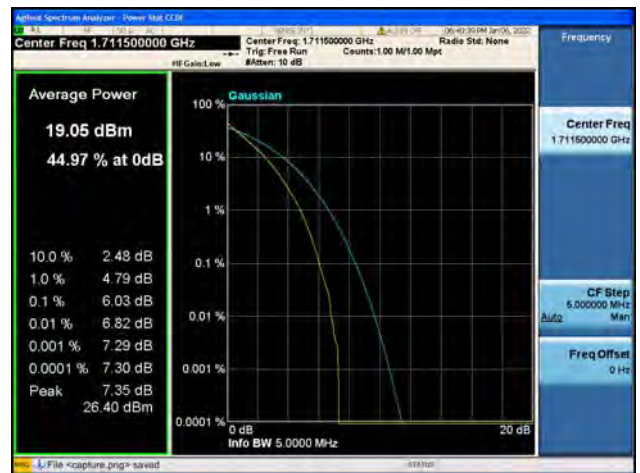
Band4 / 3MHz / Low CH / 64QAM
