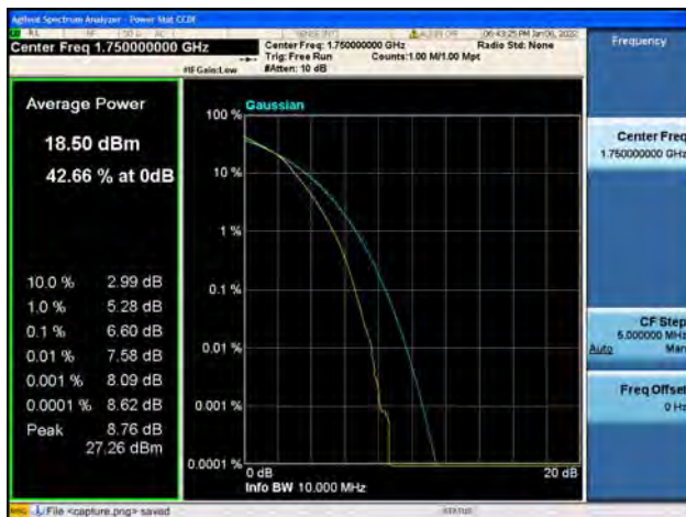
Band4 / 10MHz / High CH / 16QAM
