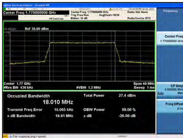
Band66 / 20MHz / High CH / 16QAM
