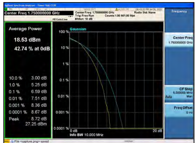
Band4 / 10MHz / High CH / 64QAM
