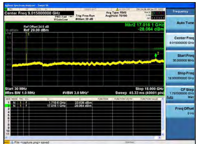
Band4 / 3MHz / Low CH / 64QAM
