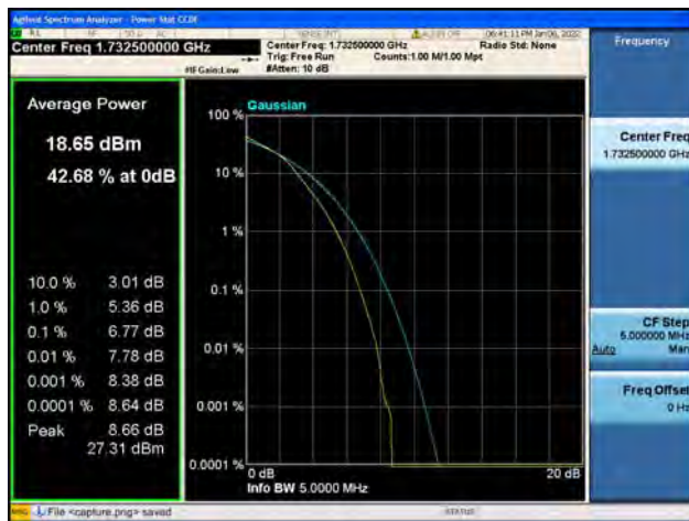
Band4 / 3MHz / High CH / 16QAM
