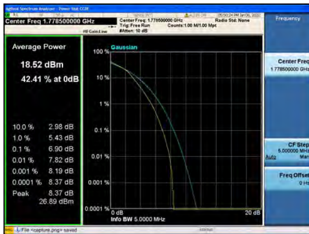
Band66 / 3MHz / High CH / 16QAM
