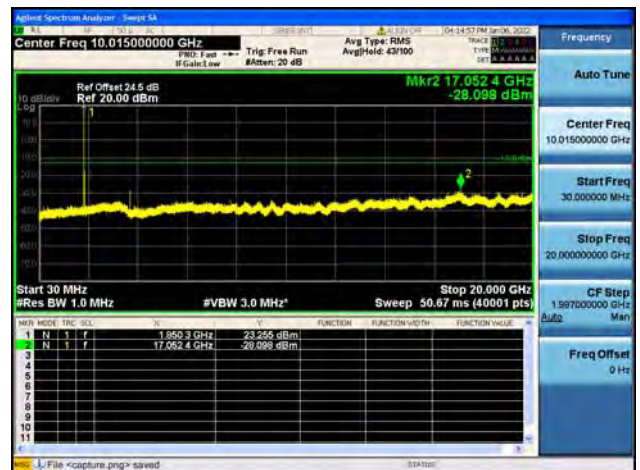
Band2 / 3MHz / Low CH / 64QAM
