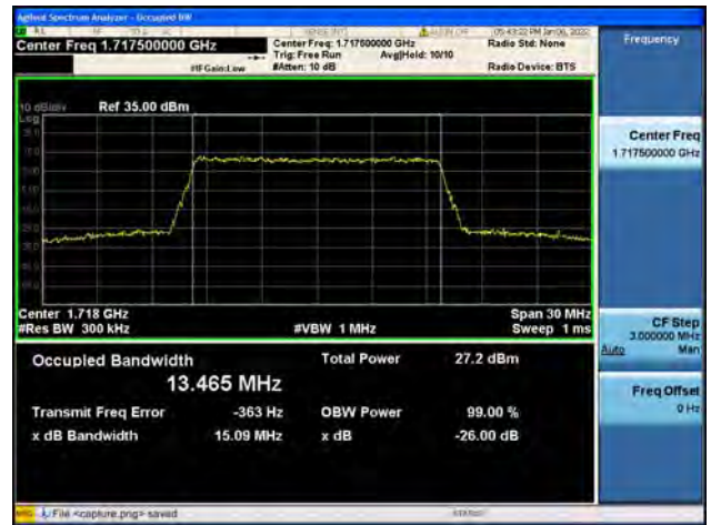
Band66 / 15MHz / Mid CH / QPSK
