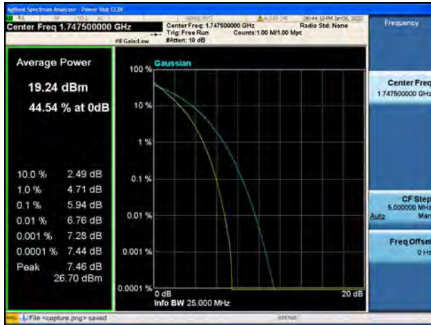
Band4 / 15MHz / High CH / 64QAM
