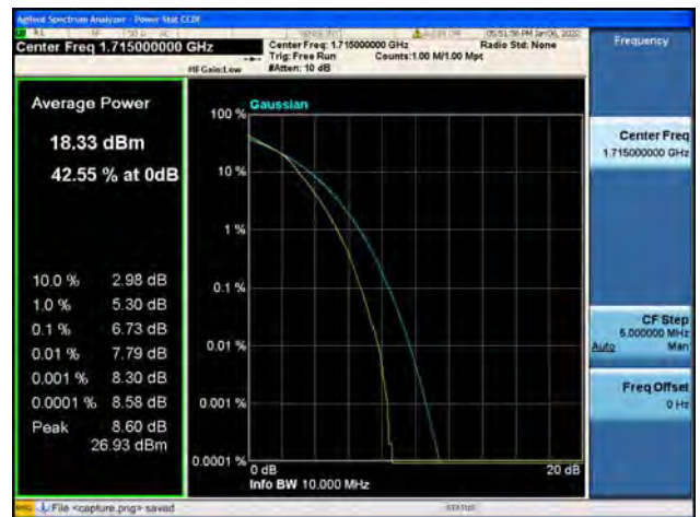
Band66 / 10MHz / Low CH / 64QAM
